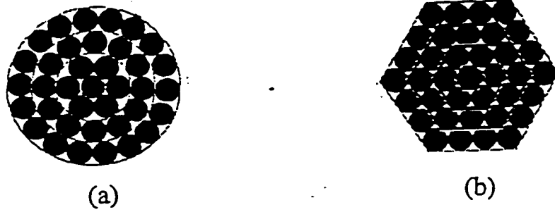
Fig 3.5 Fiber packing in yarns: (a) open-packing in circular yarns; (b) close-packing in hexagonal yarns. [2]
