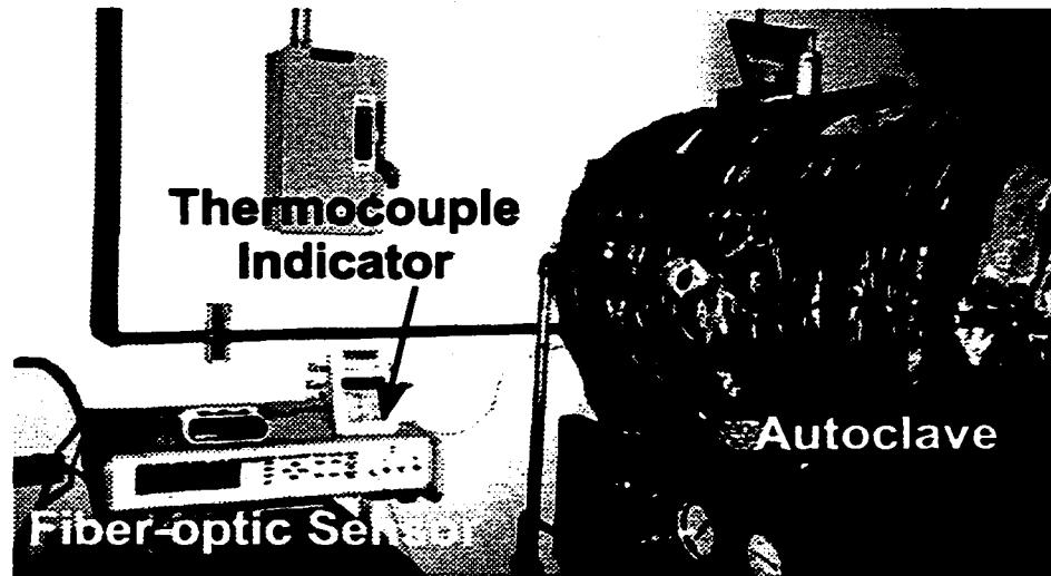
Figure 4-1 Actual in-situ fiber-optic cure monitoring system
