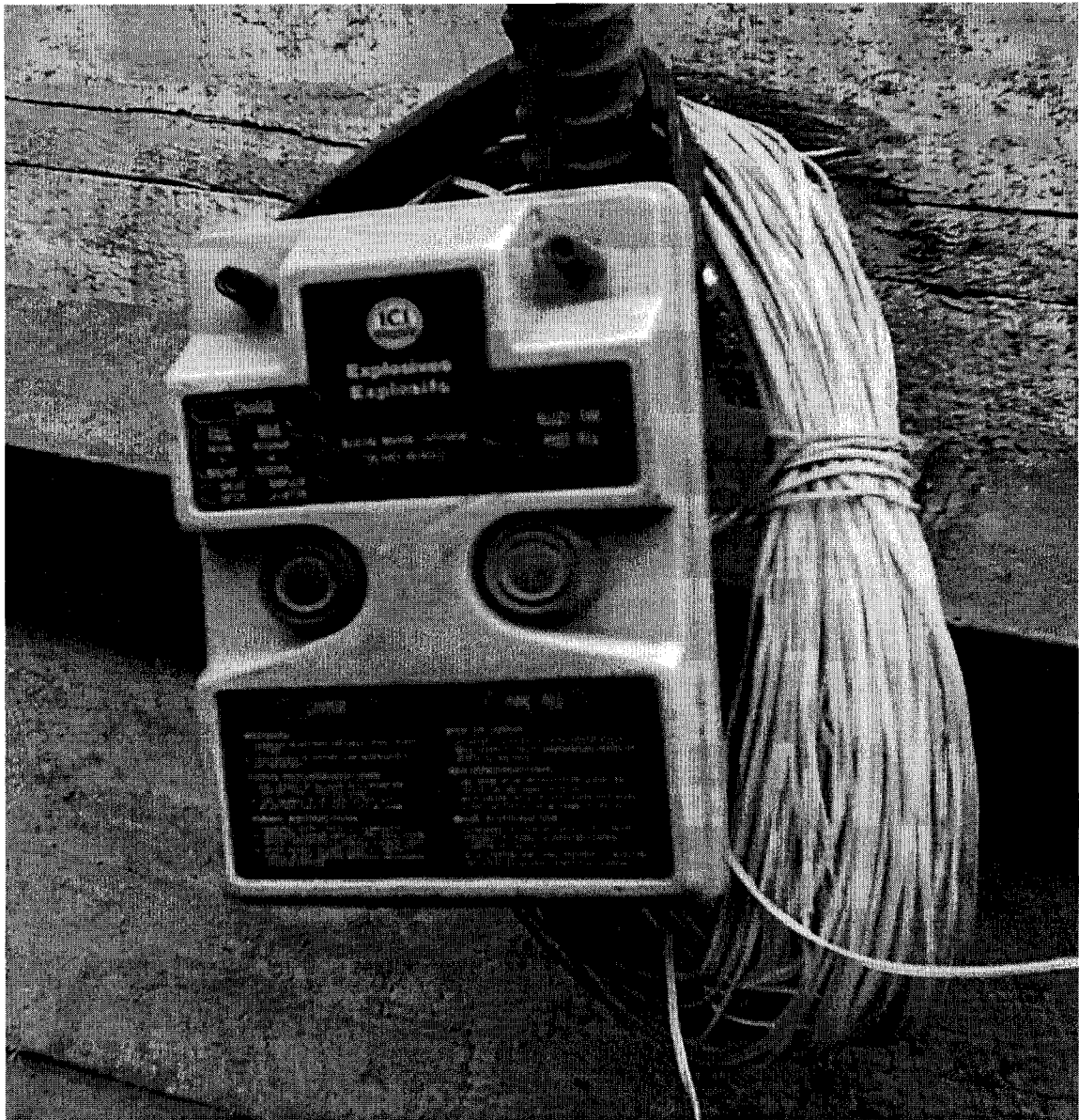
Figure 3.35 IC100 6V battery power source
