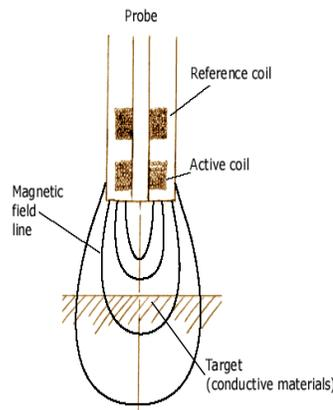
Figure 0-8 Eddy Current Technique (Efunda, 2011)
