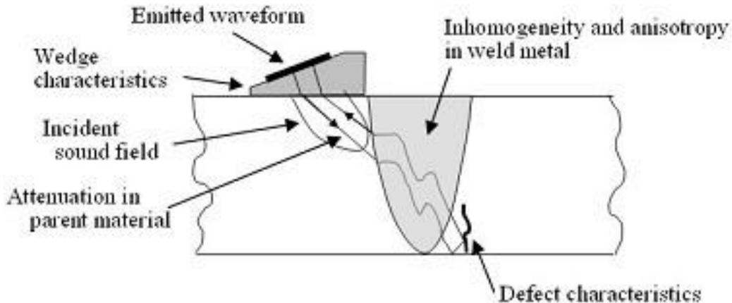
Figure 0-7 The Ultrasonic Technique (Komura, et al., 2009)
