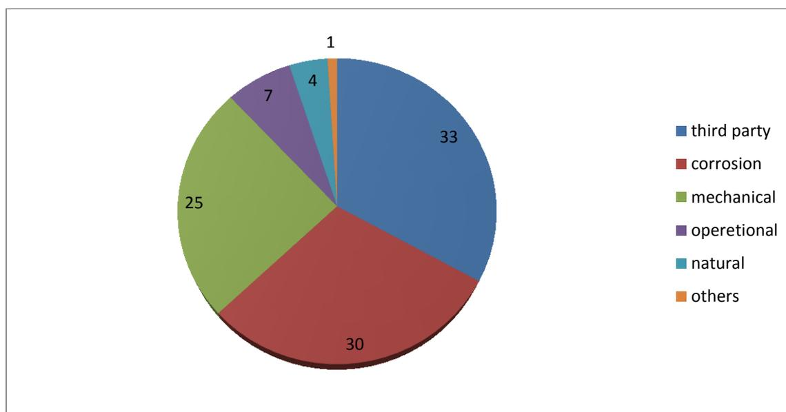
Figure 4-2 Percentage of Accidents Related to Failure Types
