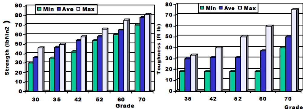
Figure 2-1 Overview of the Yield Stress and the Impact Toughness for Oil and Gas Pipeline (Hopkins, 2002)
