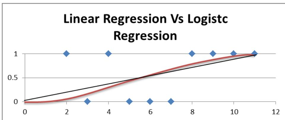
Figure 2-7 Comparison between Linear Regression and Logistic Regression
