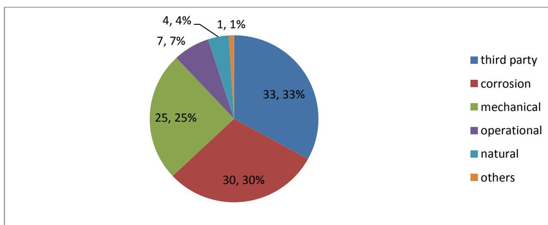
Figure 2-2 Percentages of Oil Pipeline Failure Causes (Davis, et al., 2010)
