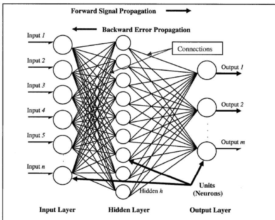
Figure 2-6 BPNN Architecture With one Hidden Layer (Barqawi, 2006)
