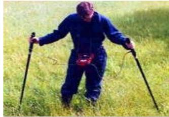
Figure 0-4 DCVG inspection and tool (Southern Cathodic Protection Company, 2007)
