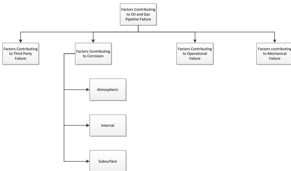
Figure 2-3 Types of factors Contributing to Pipeline Failure (Muhlbauer, 2004)
