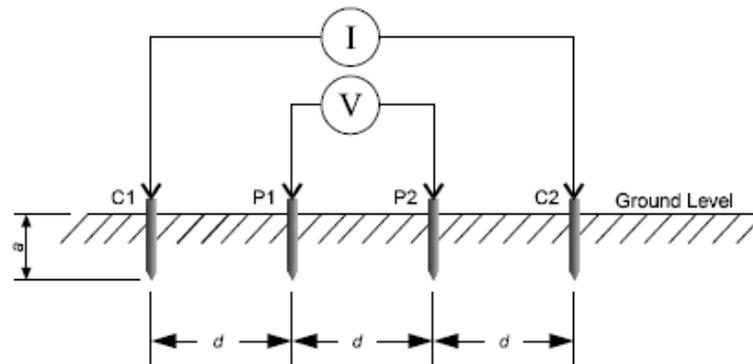
Figure 0-6 Wenner 4 Pin Test test (Lightning and Surge Technologies)
