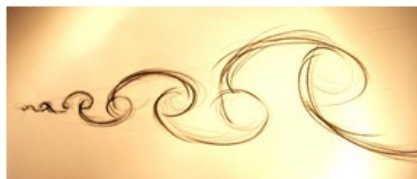
Figure 7: Sketch depicting the appearance of vortex pairing showing downstream eddies as larger and fewer in number
