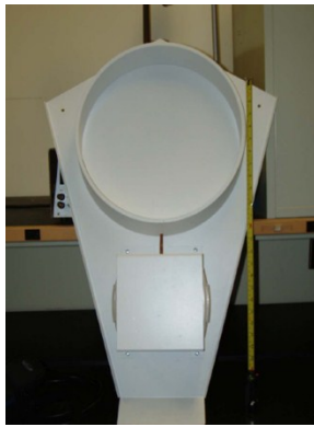
Figure 19: A plate driving rain gauge with circular collection area and concealed tipping bucket recording mechanism (photograph courtesy of National Research Council Canada)
