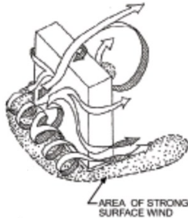
Figure 10: Air flow patterns around a rectangular building, including a depiction of the frontal vortex and recirculation zones (American Society of Heating, Refrigerating, and Air-Conditioning Engineers, Inc., 2009)
