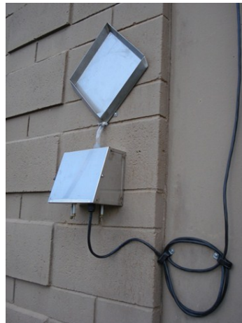
Figure 26: Photograph of a prototype of the wind-driven rain gauge deployed on a campus building
