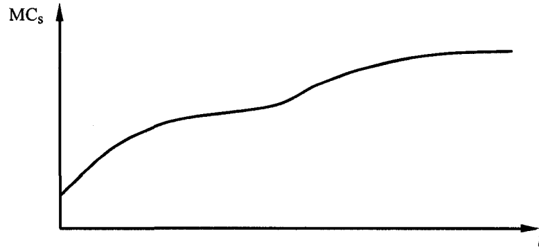
Figure 4.2. Profile of moisture state in the sheathing board
