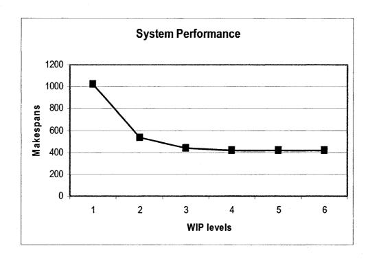
Figure 6.2: Makespan vs. WIP Level in Single CONWIP Line Example 1
