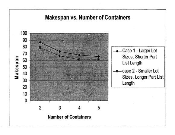
Figure 6.1: CONWIP System Performance for Different Lot Sizes
