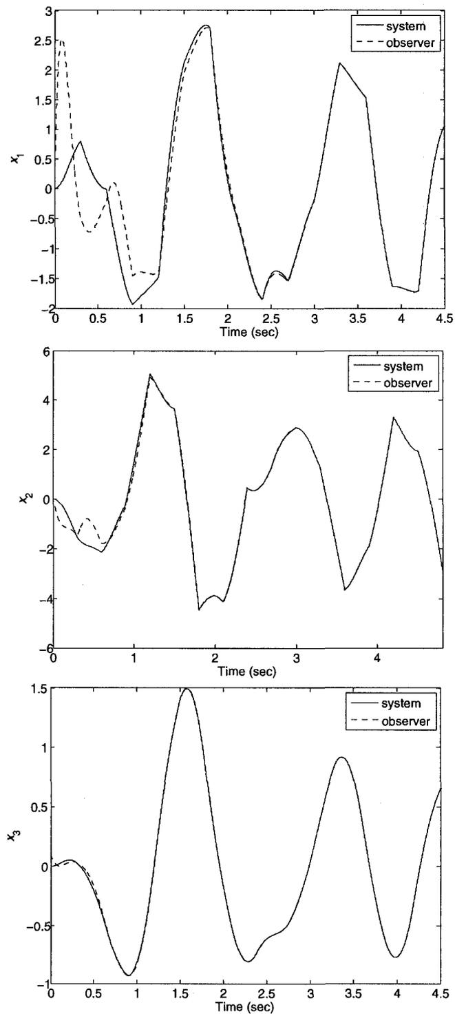
Figure 4.6: Finite time observer with  $T=0.3$
