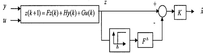
Figure 4.12: Structure of discrete finite-time observer.
