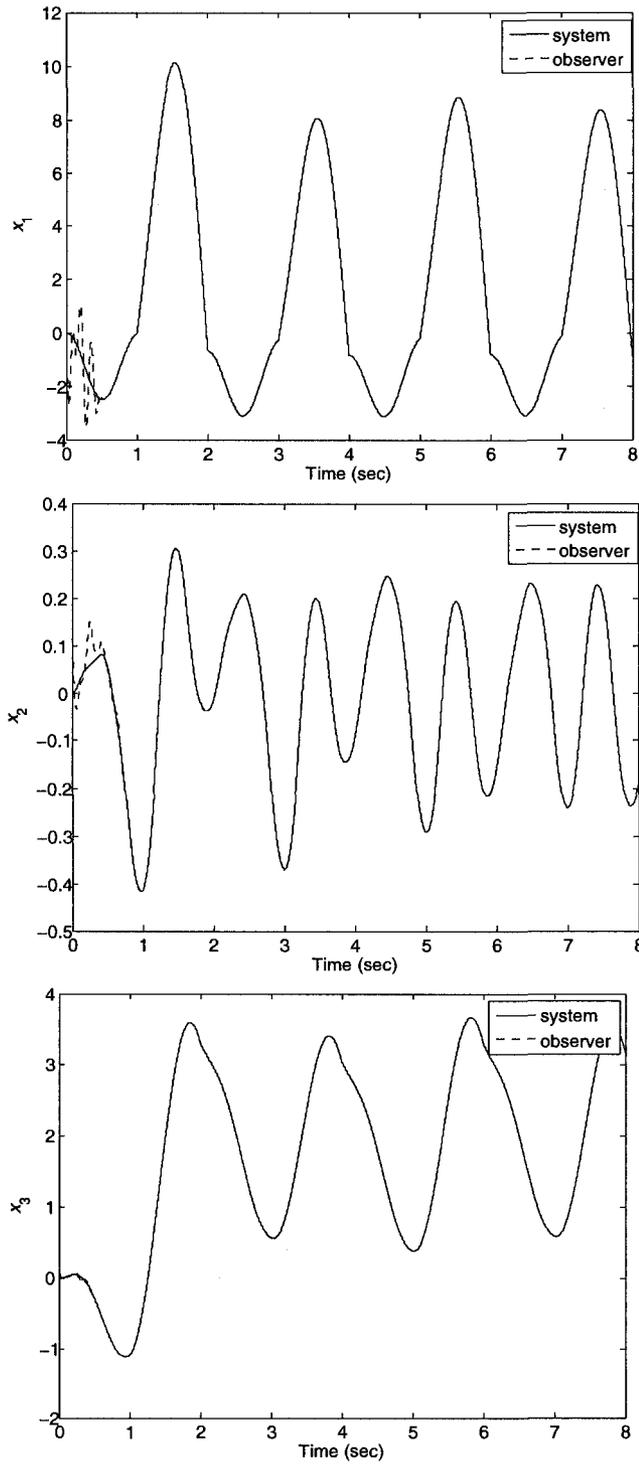
Figure 4.5: Finite time observer with  $T=0.8$
