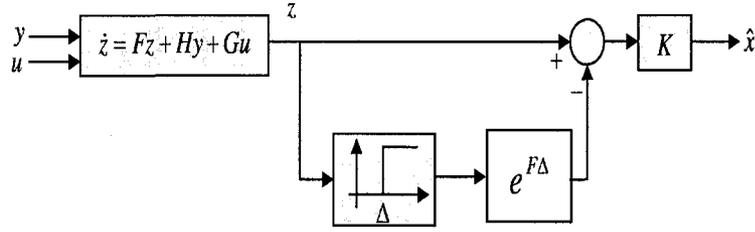
Figure 4.1: The structure of a finite-time observer [13].
