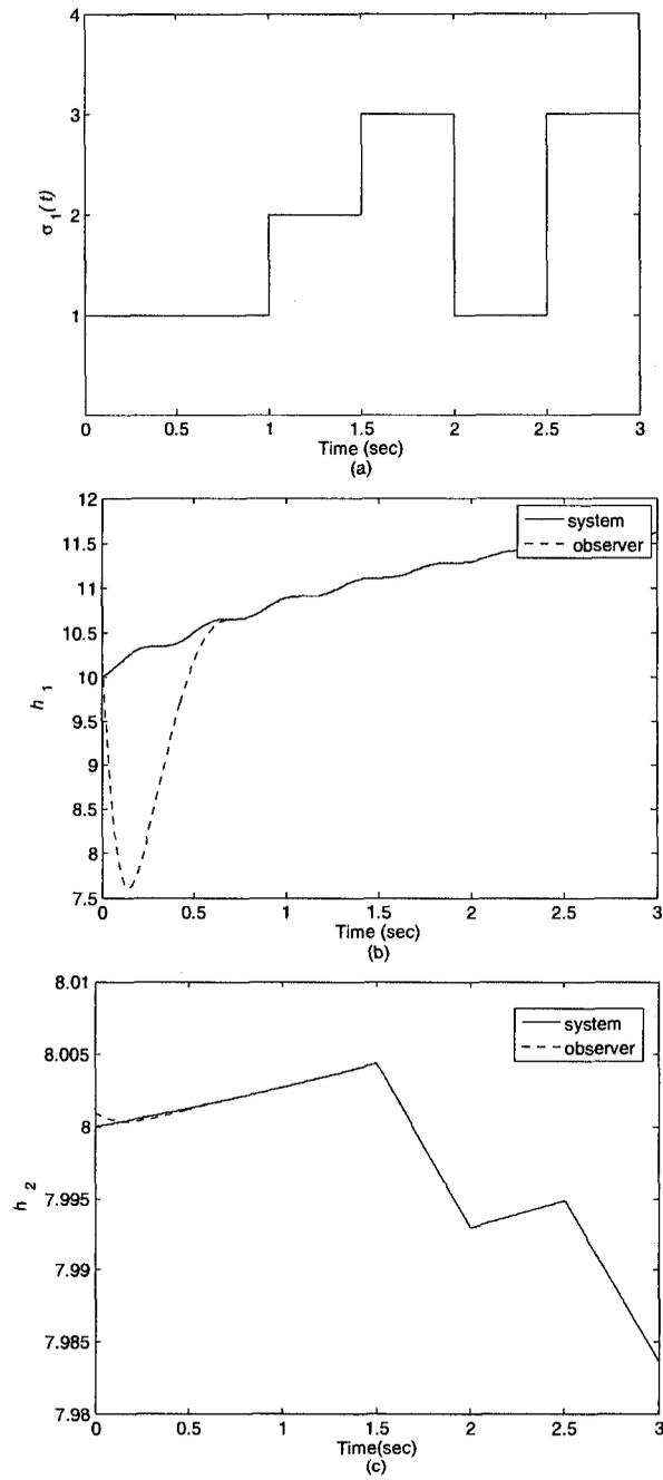
Figure 4.8: (a) Switching signal  $\sigma_1(t)$ ; (b) finite convergence time to observe  $h_1$ ; (c) finite convergence time to observe  $h_2$ .
