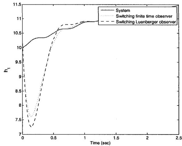
Figure 4.11: Comparison between the proposed switching finite-time observer and classic switching observer.
