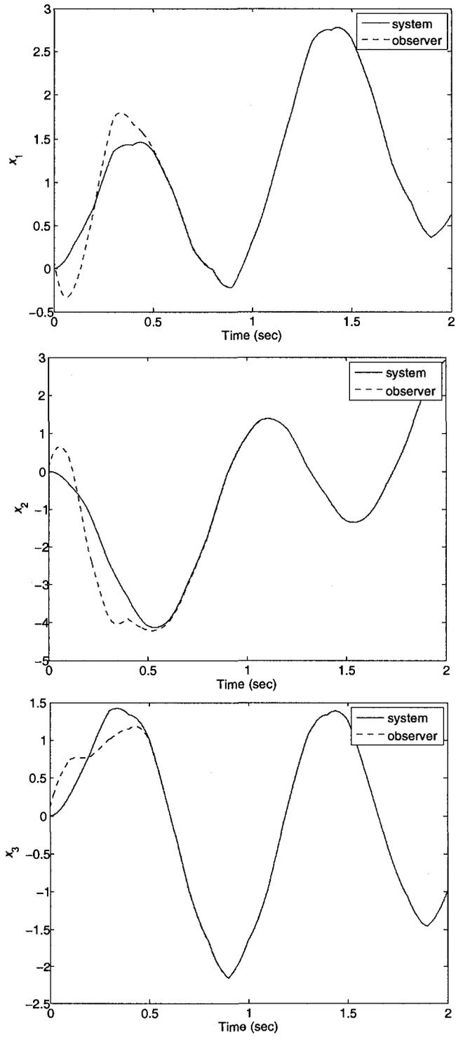
Figure 4.4: Finite time observer with  $T=0.1$
