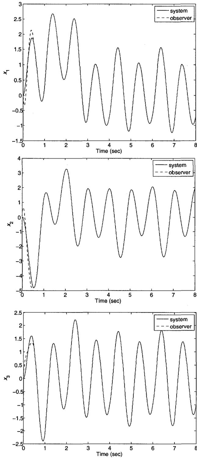
Figure 4.3: Finite time observer with  $T=0.8$
