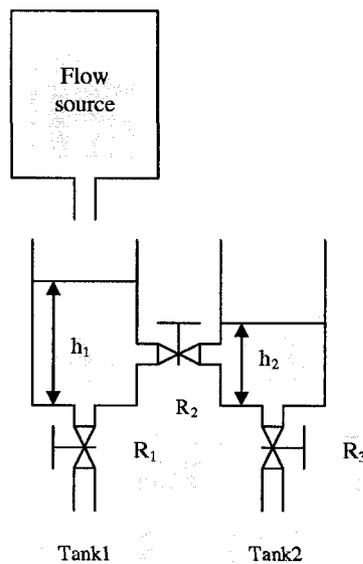
Figure 4.7: The two-tank system of Example 1.
