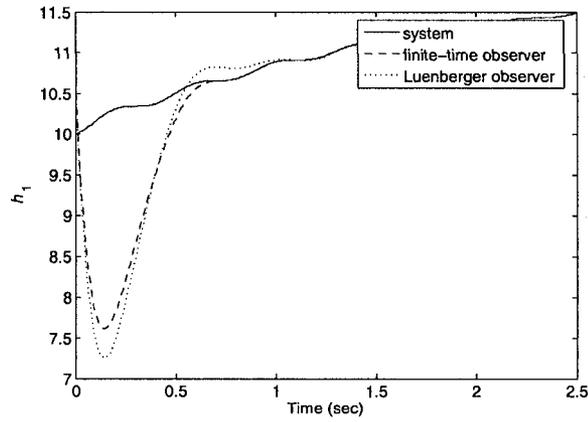
Figure 4.10: Comparison between the proposed finite-time observer and Luenberger observer.
