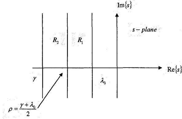
Figure 4.2: The location of the eigenvalues of the matrices  $F_i^1$  and  $F_i^2$ .
