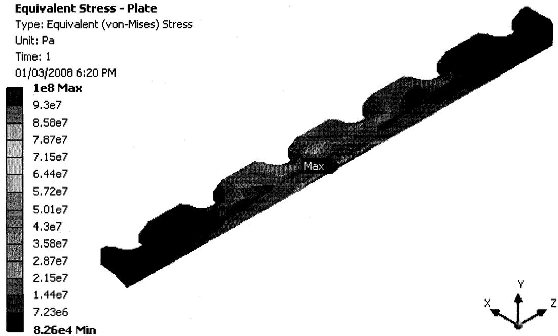
**Figure 4.15: Stress distribution in the SS plate for the 1<sup>st</sup> of week of healing**
