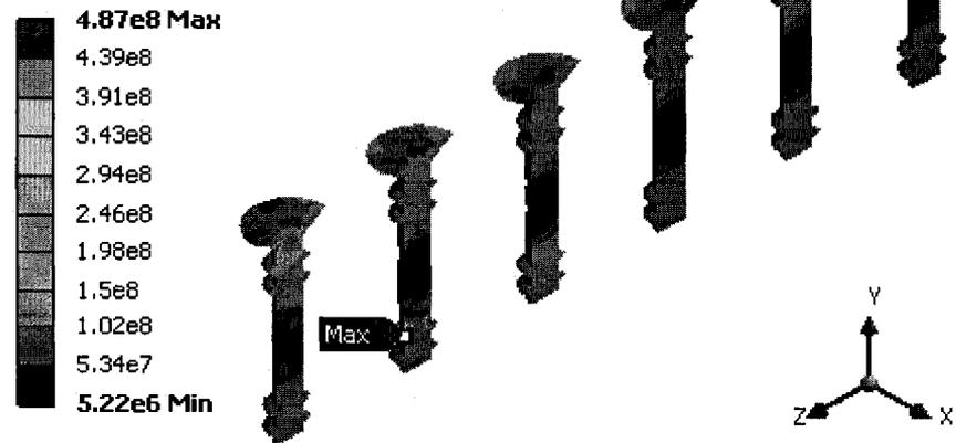
**Figure 4.45: Stress distribution in the stainless steel screws for the 8<sup>th</sup> week of healing**
