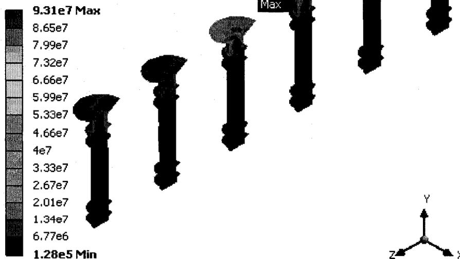
**Figure 4.8: Stress distribution in the titanium screws for the 1<sup>st</sup> week of healing**
