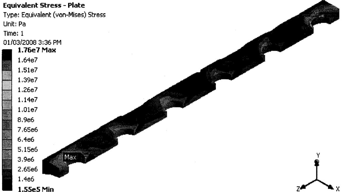
**Figure 4.6: Stress distribution in the SS plate for the 3<sup>rd</sup> week of healing**
