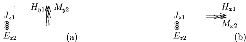
Figure A.5: Reciprocity theorem is applied to obtain the electric field E_{z2} generated by (a) a y-directed magnetic line source M_{y2} , and (b) a x-directed magnetic line source M_{x2} .
