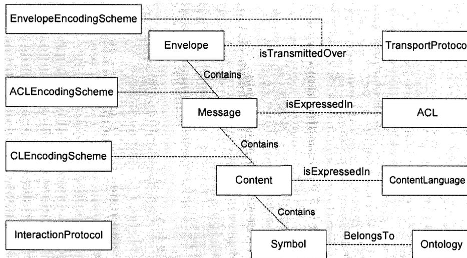
Figure 2.3 FIPA Standard: components of the communication model
