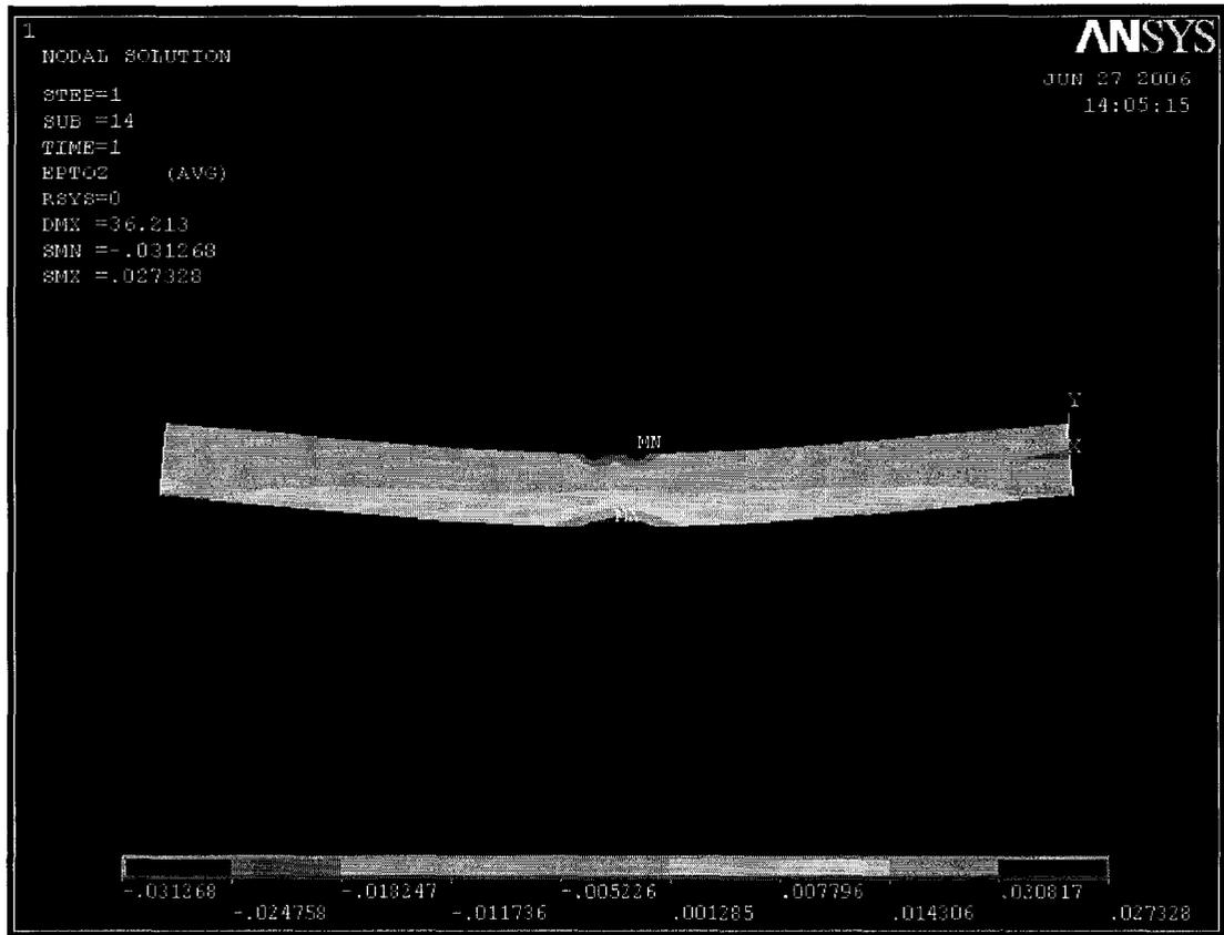
**Figure 4-3: Strain distribution in the aluminum tube**
