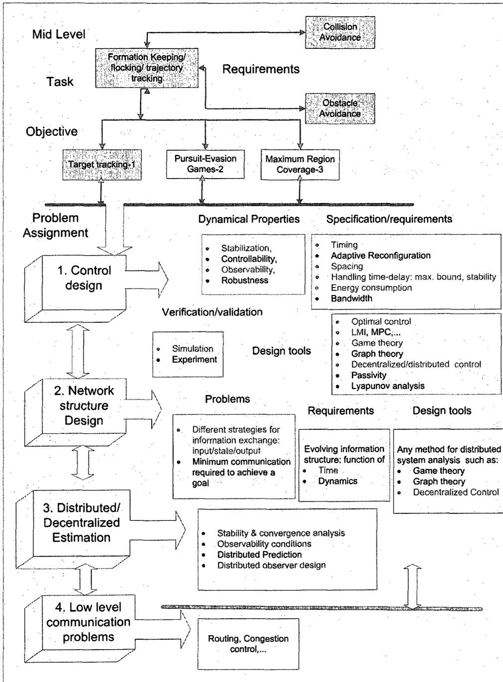
Figure 1.7: Problem assignment levels in a team design
