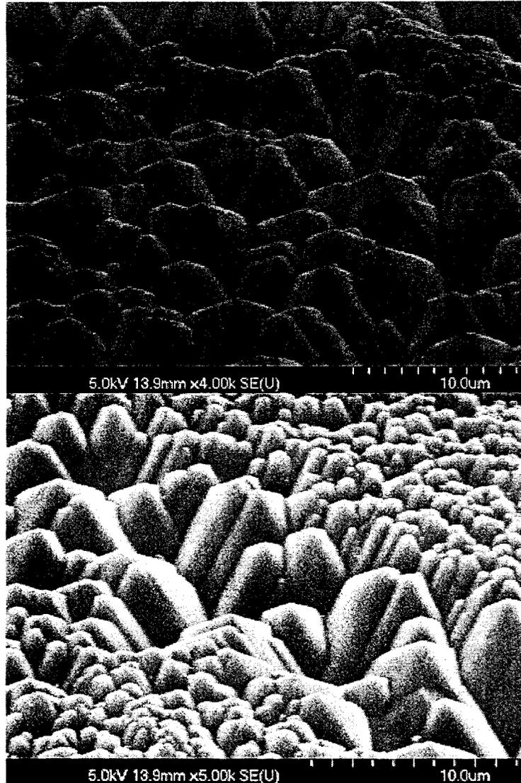
**Figure 4.17** PS obtained by electrochemically etching of n-type silicon with constant current of 85mA and anodization time of 100 seconds- tilted view (45°)-Sample#8.
