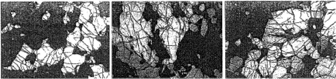
**Figure 3-8 Digitized monochrome reflected photomicrograph photos of massive Norwegian Ilmenite ore treated with microwave radiation of 2.6kW power, 2.45GHz and exposure time of 0, 30 and 60 sec respectively from left to right (Kingman et al., 1998).**
