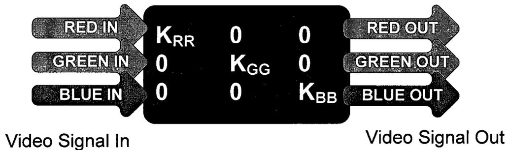
**Figure 3.21: LED pixel correction coefficients for W color and luminance methodology**
