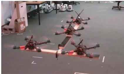
(c) Cooperative object transportation using quad-rotors. Work done at GRASP Lab, University of Pennsylvania.
