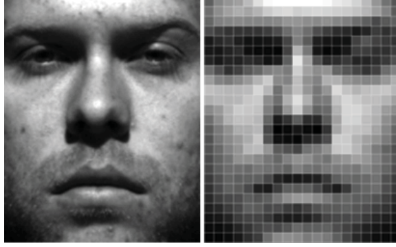
Figure 3.6: Resizing the image to reduce the computation time. The pixels of the right image are 100 times larger than the pixels of the left image.
