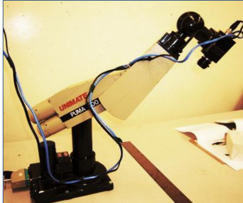
Figure B.6 PUMA 260 with a camera mounted on the End-Effector
