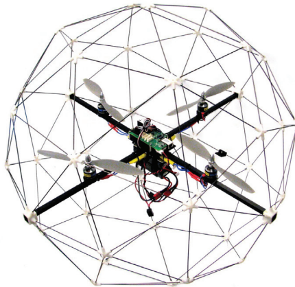
Figure 3.7: The Qball-X4 quadrotor UAV (Quanser, 2010)
