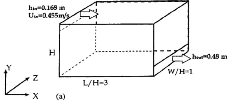
Figure 2.6 The sketch of empty room with ventilation [51]
