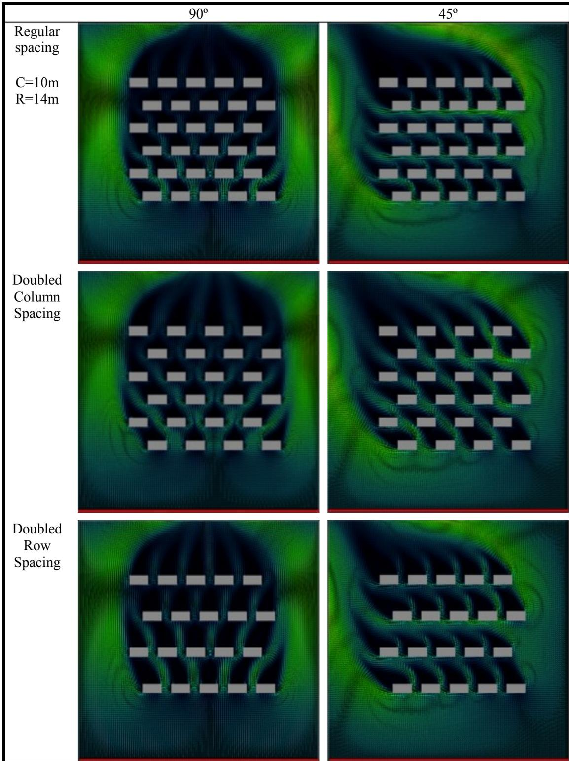
Figure 5.16 Screenshots of FFD simulation on staggered building arrangement
