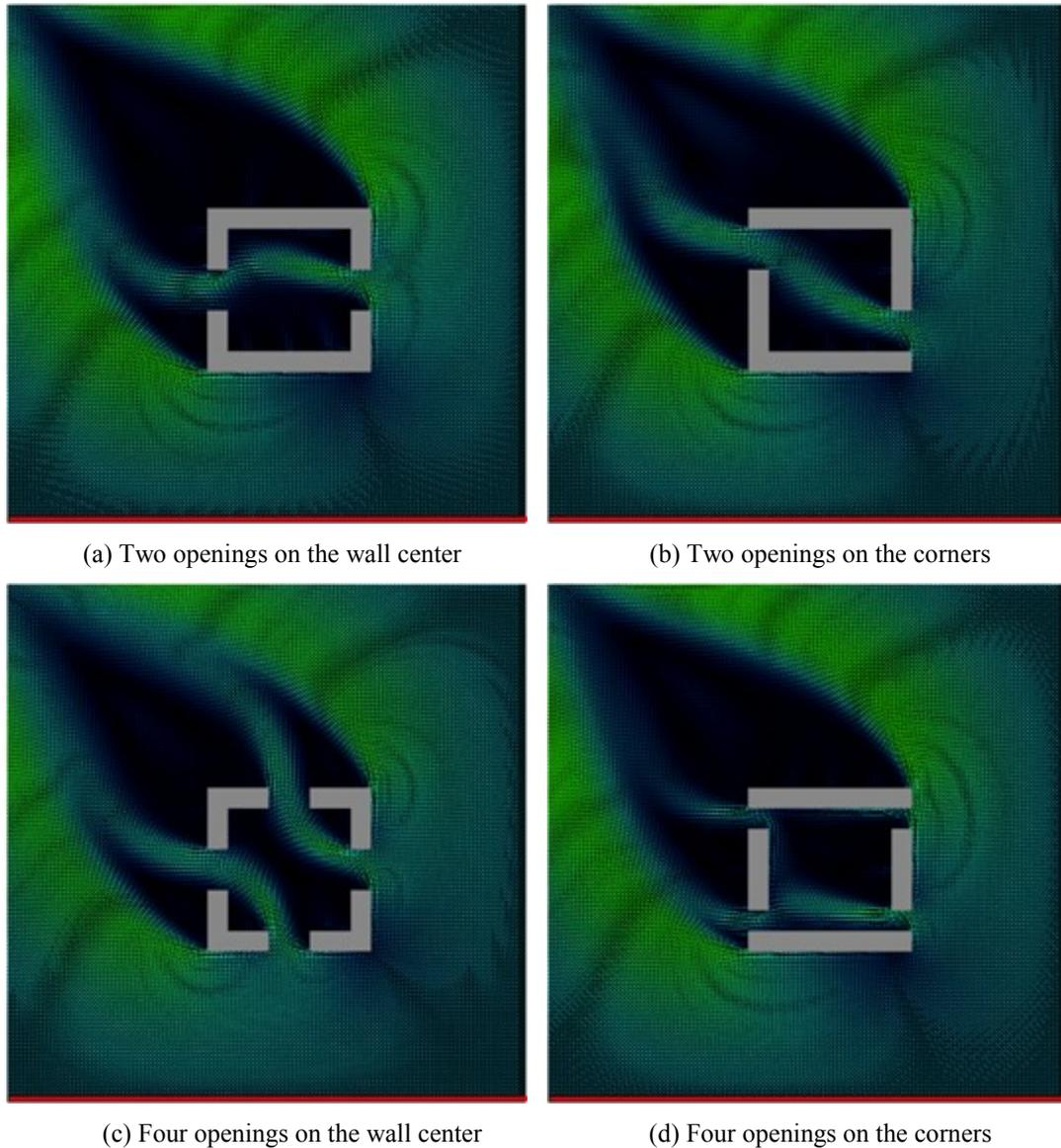
Figure A.1 Screenshots of simulation on four enclosed building pattern at wind speed 6m/s, orientation 45°
