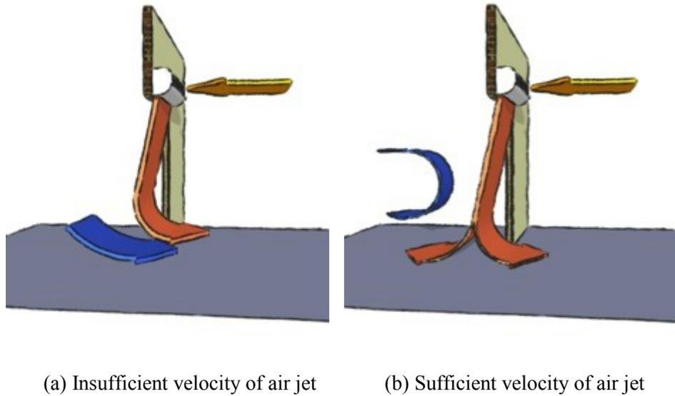
Figure 5.1 Air curtain working modes illustration
