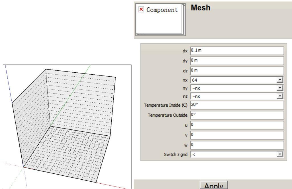
Figure A.2 Mesh (left) and its configuration dialogue box (right)
