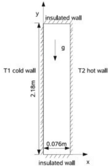
Figure 2.8 Schematic of a natural convective tall cavity [53]
