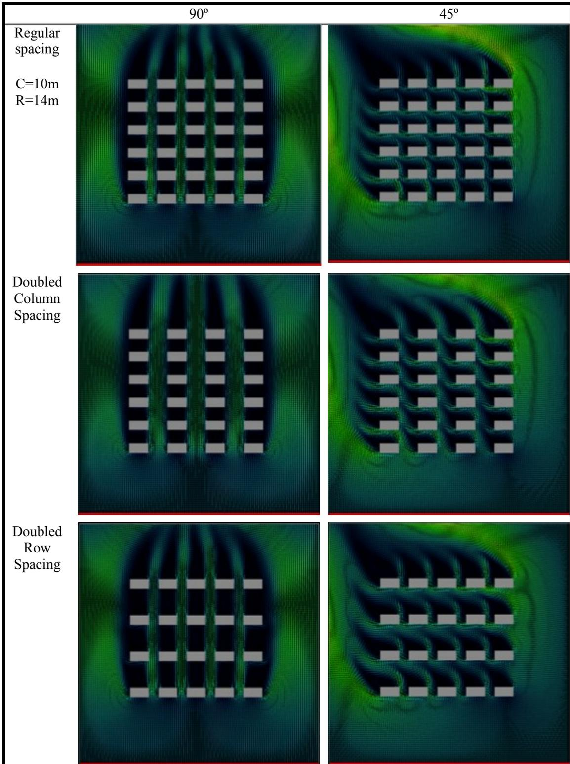
Figure 5.15 Screenshots of FFD simulation on aligned building arrangement
