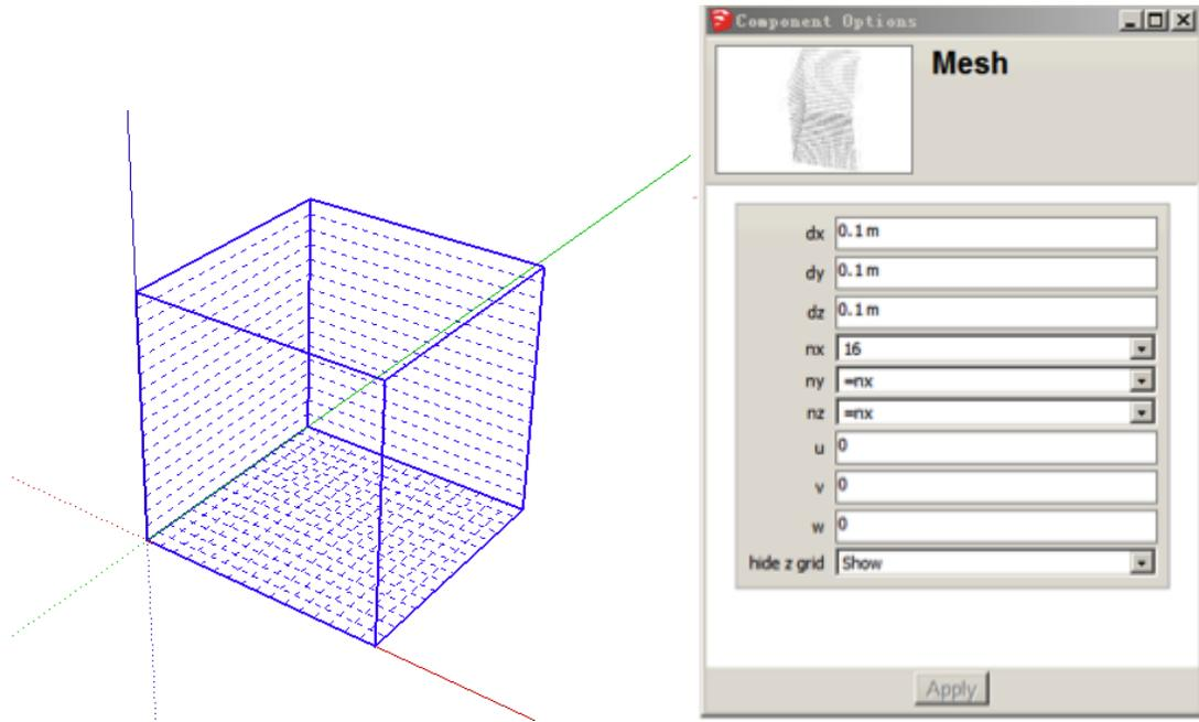
Figure 3.7 FFD SketchUp plug-in grid creating screenshot and input dialogue window
