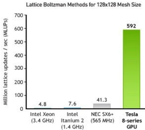
Figure 2.2 Comparison on solving CFD with Lattice Boltzman method between GPU and CPU
