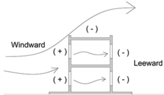
Figure 5.11 Schematic diagram of wind pressure on building
