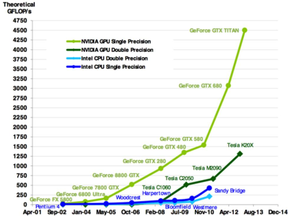
Figure 1.2 Floating-point operations per second of the CPU and GPU [30]
