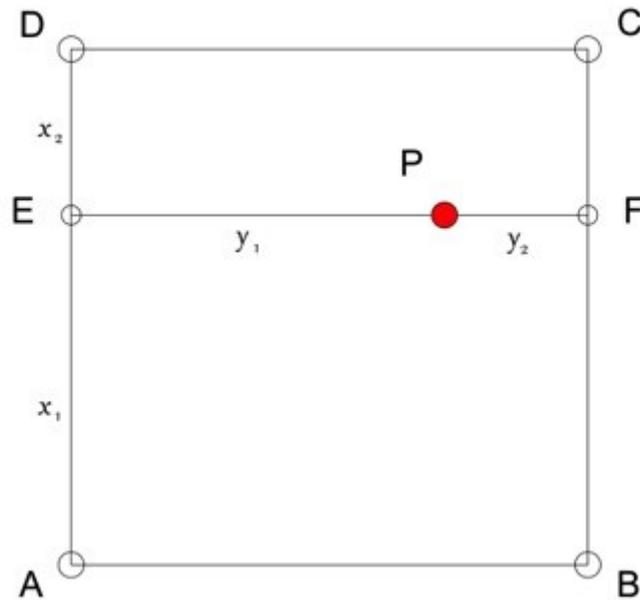
Figure 3.2 Two-dimensional linear interpolation method
