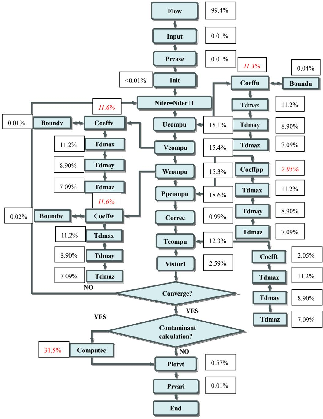
Figure 4.3 Percentile computing time for each function of the CFD module of CONTAM after the profiling in the case of the five-zone office suite with a grid resolution of  $42 \times 24 \times 24$  ( $x \times y \times z$ )
