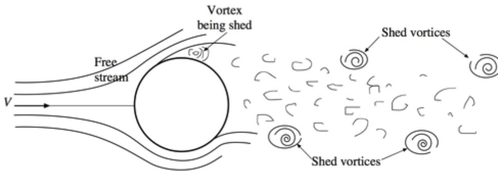
Figure 4.7 von Kármán vortex street phenomenon from a cylinder [68]
