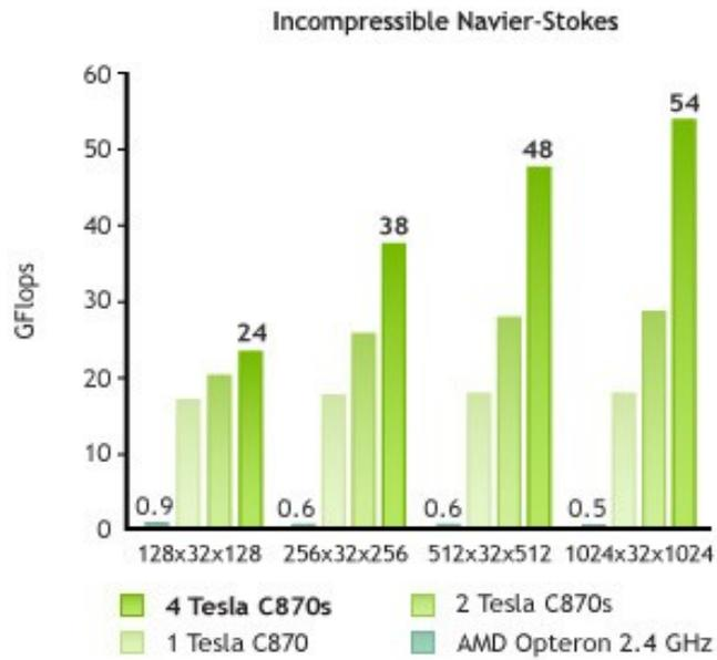
Figure 2.1 Comparison on solving CFD with incompressible Navier-Stokes method between GPU and CPU [39]
