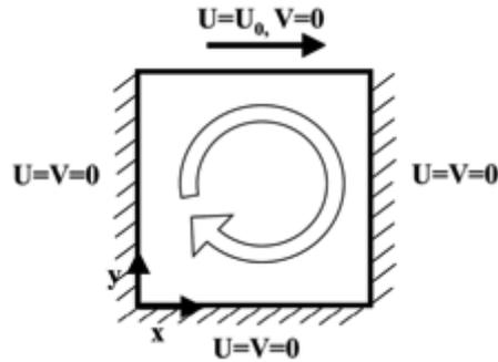
Figure 2.7 Scheme of the flow in a lid-driven cavity case [52]
