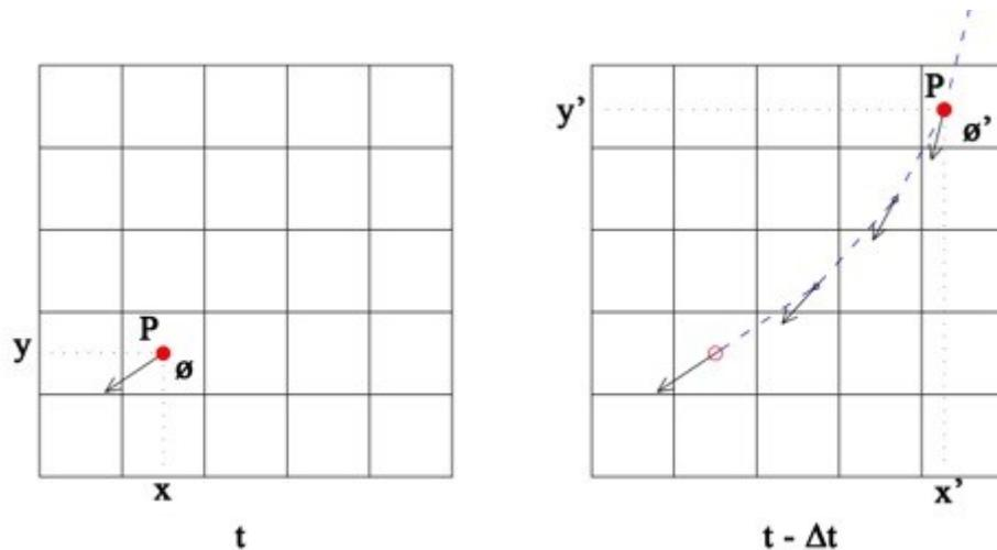
Figure 3.1 Two-dimensional illustration of Semi-Lagrangian method
