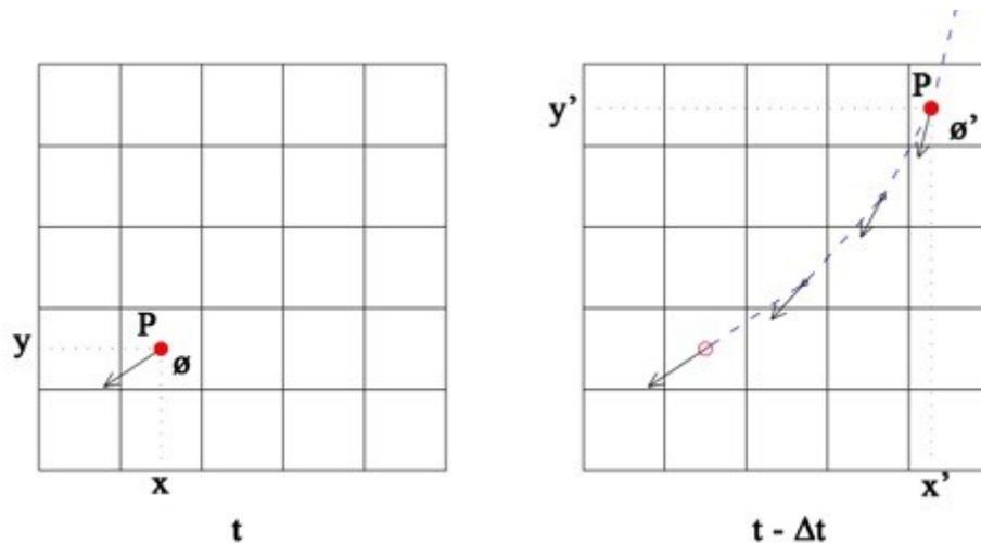
Figure 3.1 Two-dimensional illustration of Semi-Lagrangian method
