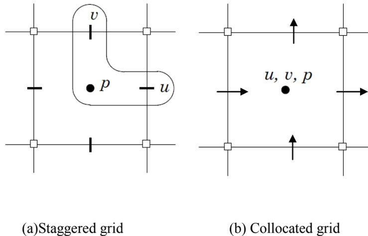
Figure 3.3 Staggered grid and Unstaggered (or collocated/cell-centered) grid (u and v are the velocity components in x and y directions, and p is the pressure) [60].
