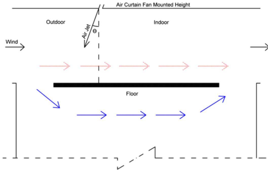
Figure 5.2 Sketch of 2D Air curtain case
