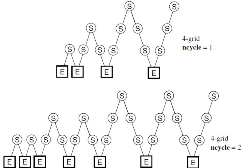
Figure 3.4 The calculation structure for the full multigrid (FMG) method in the new FFD solver. Starting on the coarsest grid, the FMG interpolates and then refines the solution onto finer grids. E means exact solution on the coarsest grid and S means smoothing [63].
