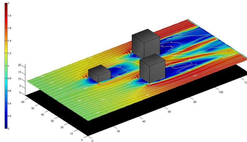
Figure 2.3 Snapshot of velocity magnitude and streamlines of urban domain simulation on GPU
