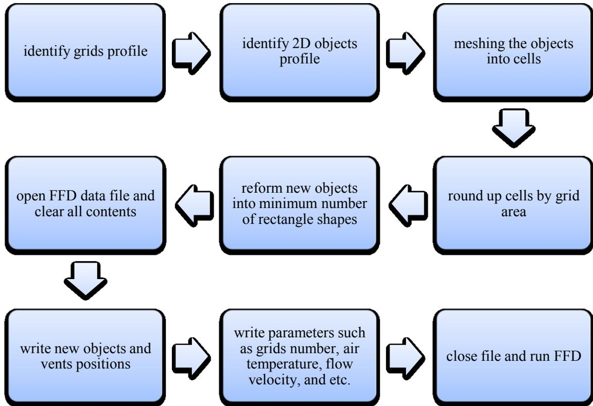
Figure 3.8 Process of converting SketchUp model information into FFD readable data
