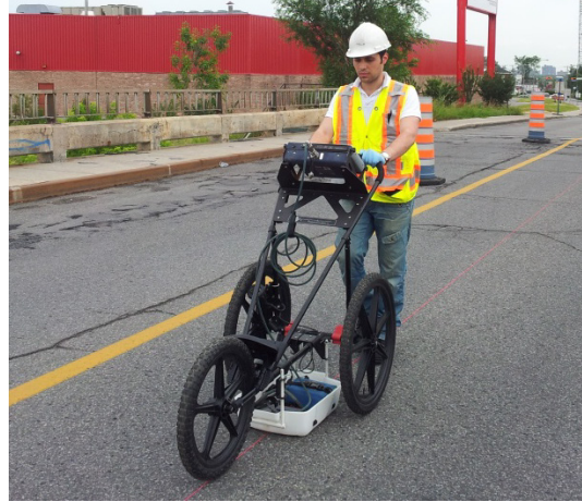
Figure 42: Wheel Mounted GPR System
