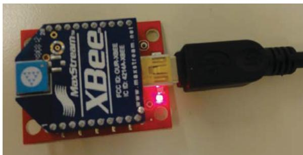
Figure 4.4: Xbee connected to the server computer.
