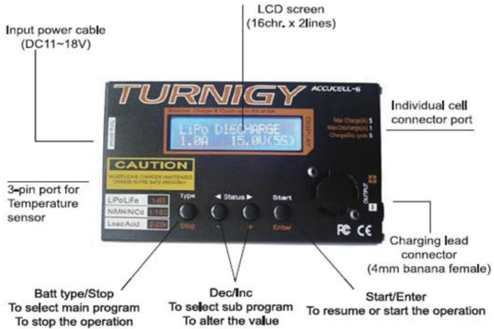
Figure 4.9: Turnigy Accucell-6 charger 9.
