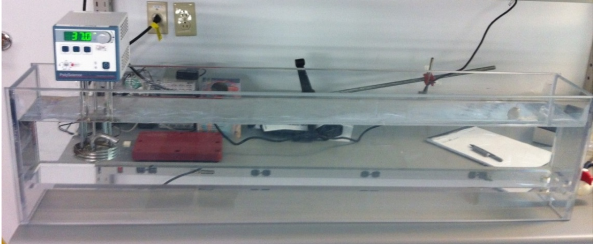
Figure 3.6 Warm water bath with thermal circulating water pump.
