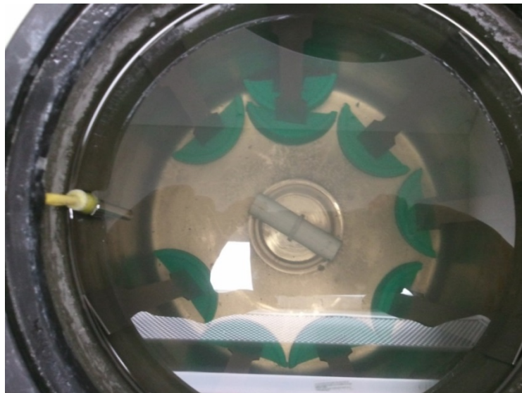
Figure 3.5 Samples submerged in isopropyl alcohol 99% cryo bath.
