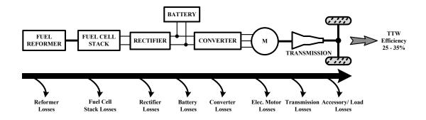
Fig. 1-4 Schematic diagram of fuel cell vehicle drivetrain
