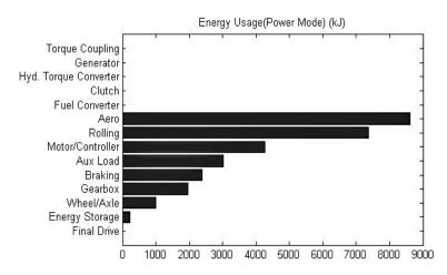
Fig. 2-11 EV total loss distribution (motoring mode) over driving cycle
