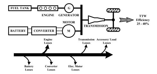
Fig. 1-3 Schematic diagram of parallel hybrid electric vehicle drivetrain
