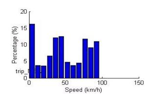
Fig. 2-3 Time percentage over Speed pattern for vehicles under study
