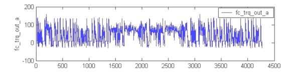
**Fig. 2-4** above: time-aligned vehicle driving speed. Below: engine torque delivery Figure 2-4 gives the IC engine torque achieved through the driving cycle, aligned with delivered speed. It is clear that, the highest achieved torque demands are associated with acceleration.
