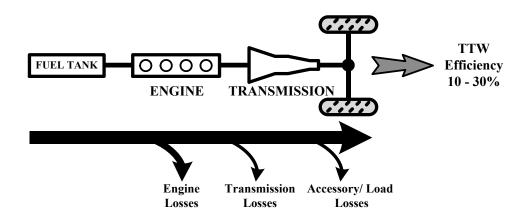
Fig. 1-2 Schematic diagram of gasoline vehicle drivetrain
