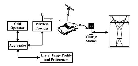
Fig. 4-2 Schematic diagram of V2G connection
