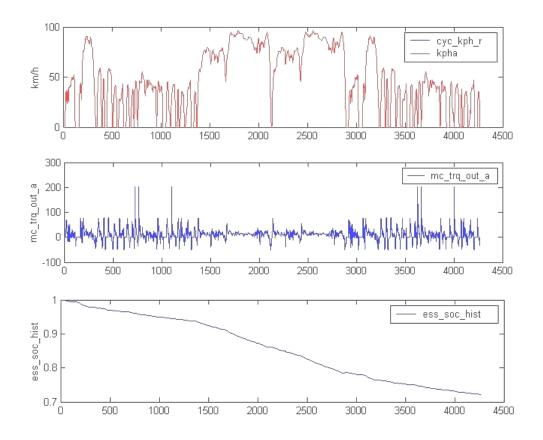
**Fig. 2-8** a. above: drive cycle, b. middle: EV simulated torque delivered by motor over drive cycle (negative during regenerative braking), c. below: state of Li-ion battery
