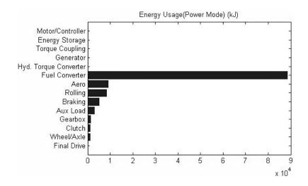
Fig. 2-7 ICE vehicle total loss distribution (powering mode) over drive cycle
