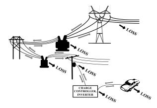
Fig. 4-4 Energy transmission and conversion losses
