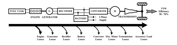
Fig. 1-5 Schematic diagram of series plug-in hybrid electric vehicle drivetrain
