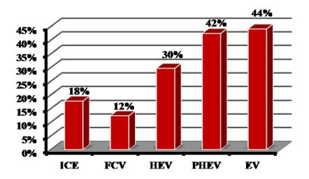
Fig. 2-12 WTW efficiency of different drivetrains
