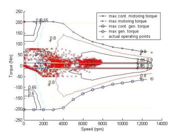
Fig. 2-9 Traction motor operating points
