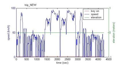
Fig. 2-2 Simulated multiple drive cycle
