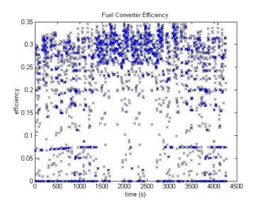
Fig. 2-6 ICE conversion efficiency during driving schedule
