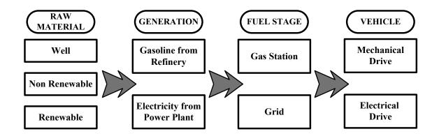
Fig. 1-1 Schematic diagram of different stages in WTW efficiency analysis
