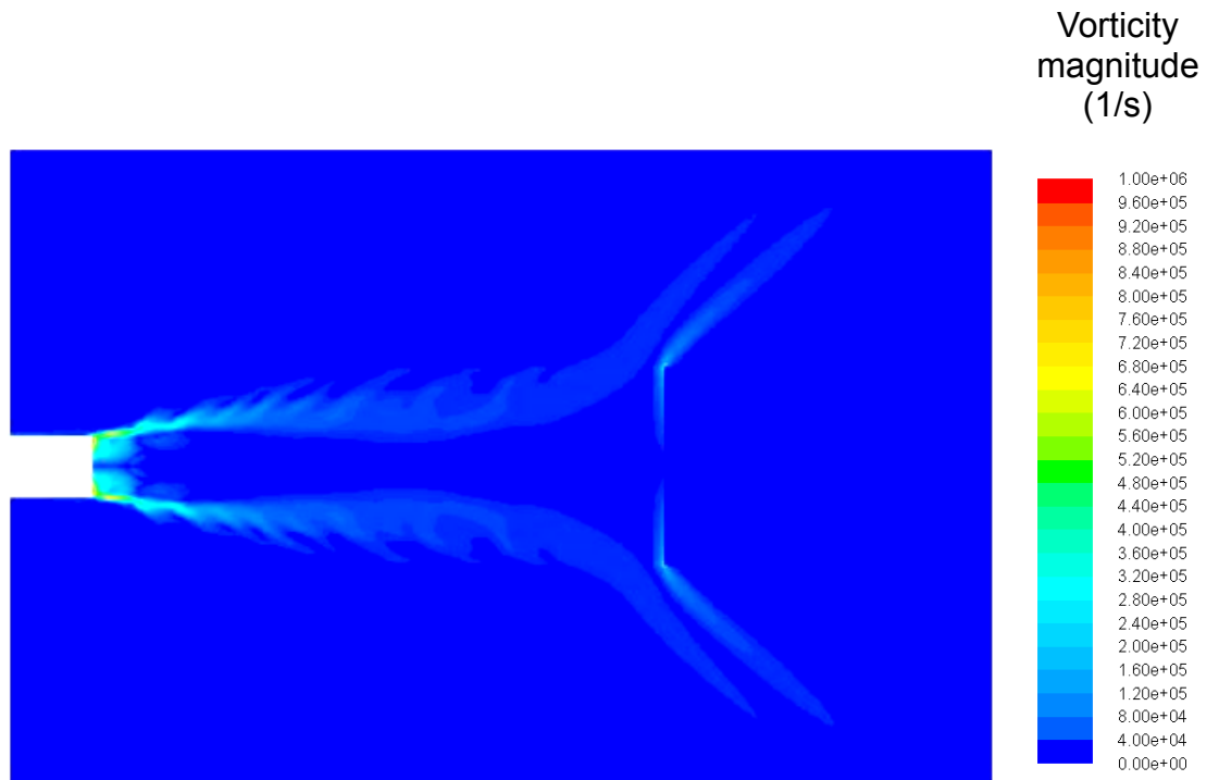
Figure 4.2 Preliminary result of the effect of substrate on the main flow, stand-off distance of 6cm, vorticity magnitude (1/s)
