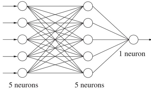
Figure 4.9: The schematic structure of the best network trained with Algorithm 2 for spindle vibration signals.
