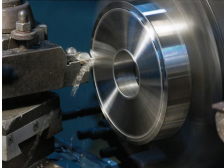
Figure 1.1: Turning operation [2].
