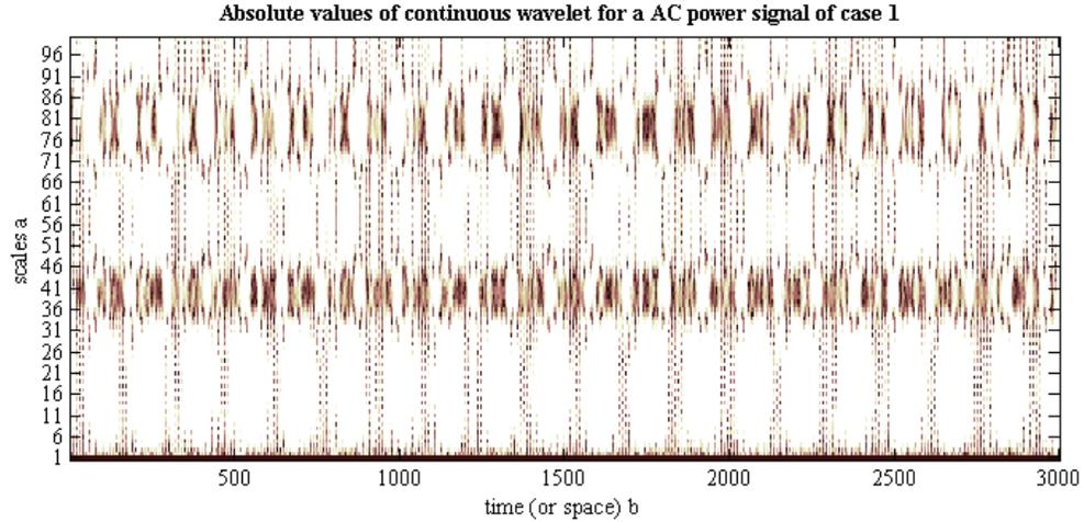
Figure 4.6: Continuous wavelet transform of a AC power signal.
