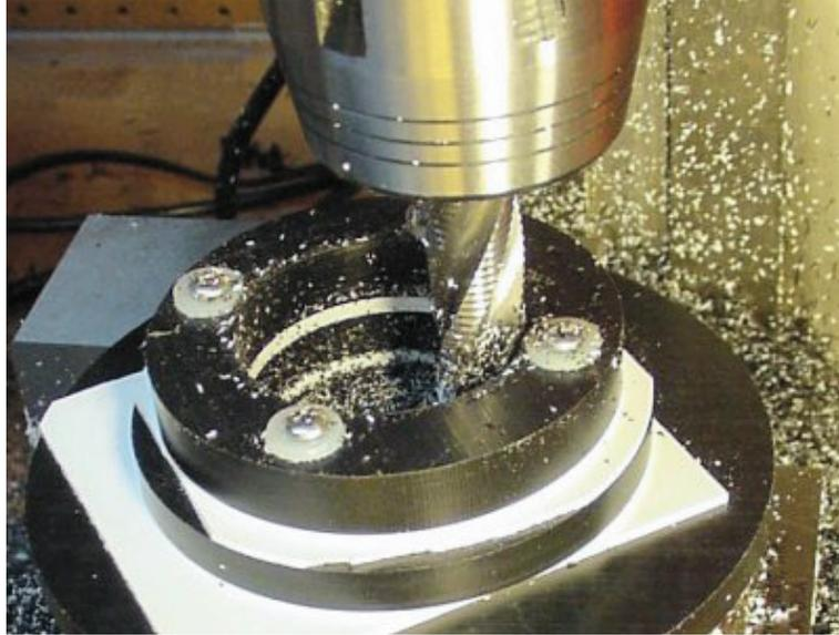
Figure 1.3: End milling operation [6].
