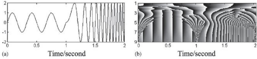
Figure 3.1: Continuous wavelet transform: A typical signal (a) and its wavelet phase map (b) (at the time of 1 s, the signals frequency changed and started to increase with time) [96].
