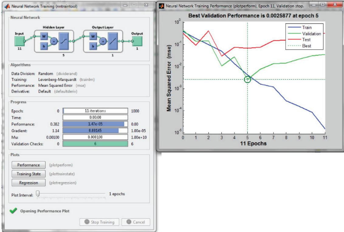
Figure 4.5: The trend of network training with Algorithm 1 for spindle vibration signals.
