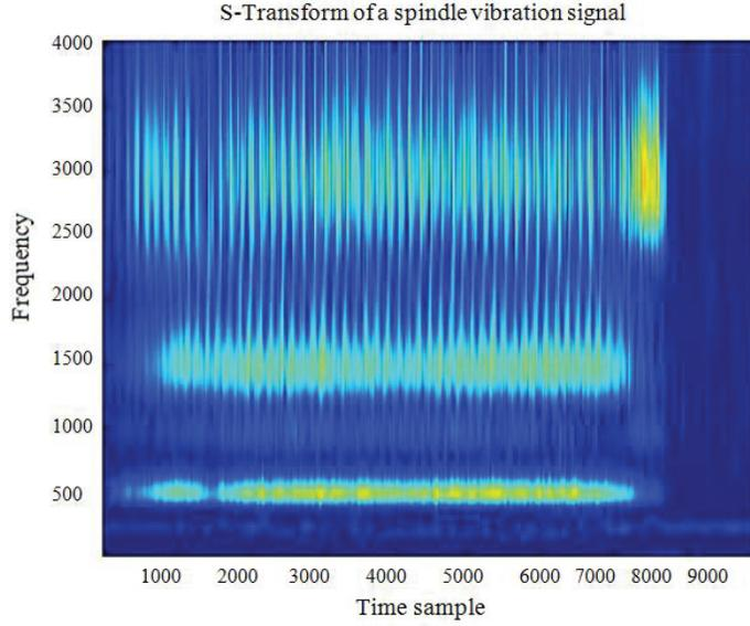
Figure 4.13: wide range frequency S-Transform analysis for a spindle vibration signal.
