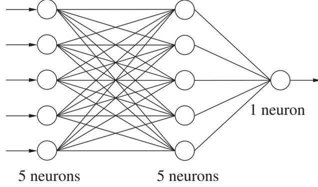
Figure 4.14: The schematic structure of the best network trained with Algorithm 4 for AC power signals.
