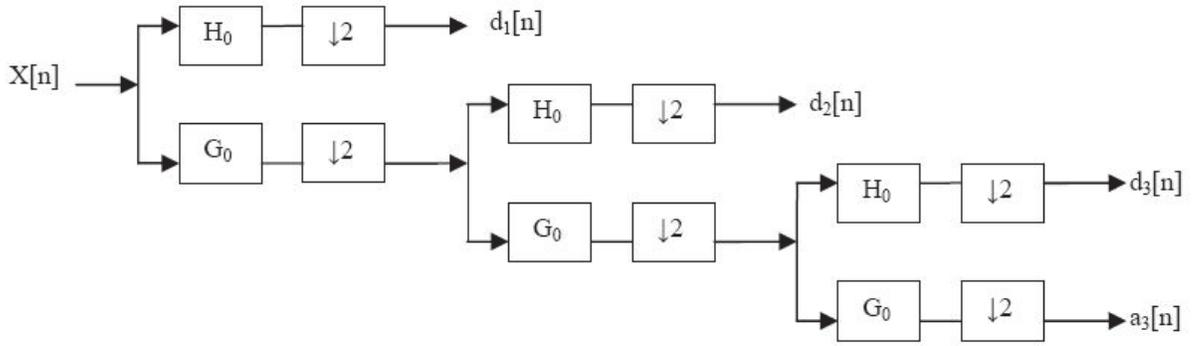
Figure 3.2: Three-level wavelet decomposition tree [99].
