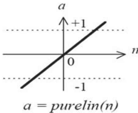
Figure 3.8: Transfer function of a neuron: purelin [114].
