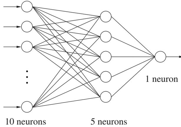
Figure 4.16: The schematic structure of the best network trained with Algorithm 5 for table vibration signals.
