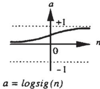
Figure 3.6: Transfer function of a neuron: logsig [114].
