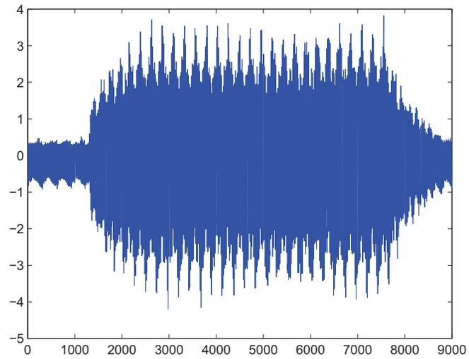
Figure 2.3: Spindle motor current signal (AC).
