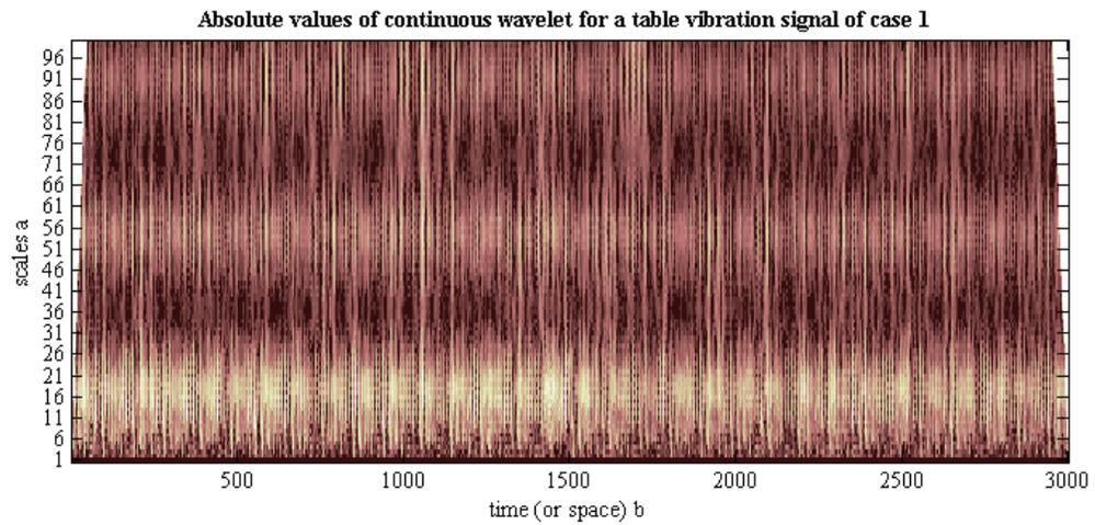
Figure 4.7: Continuous wavelet transform of a table vibration signal.
