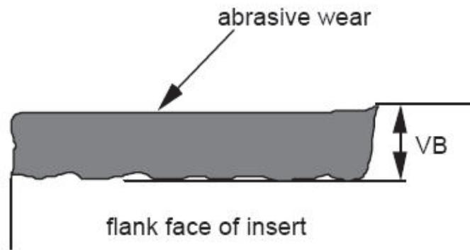
Figure 2.2: Tool flank wear (VB) as it is seen on the insert [90].
