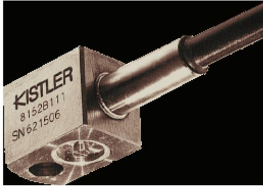
Figure 1.10: AE sensor [57].
