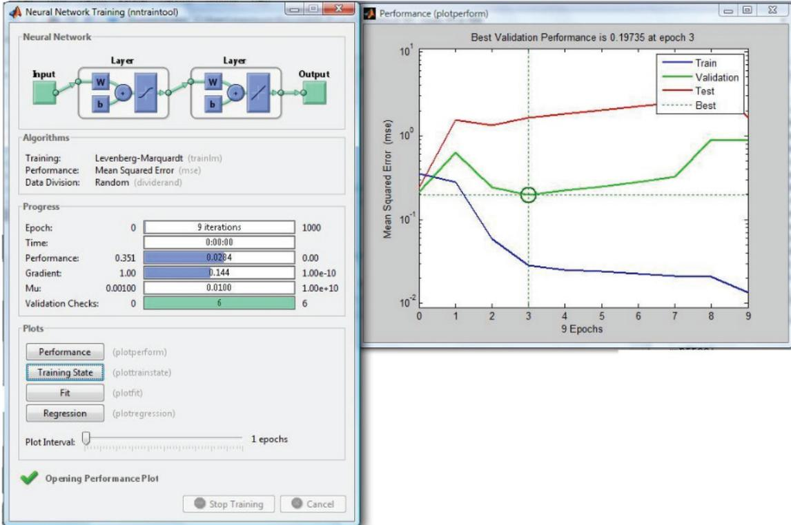
Figure 4.10: The trend of network training with Algorithm 2 for spindle vibration signals.
