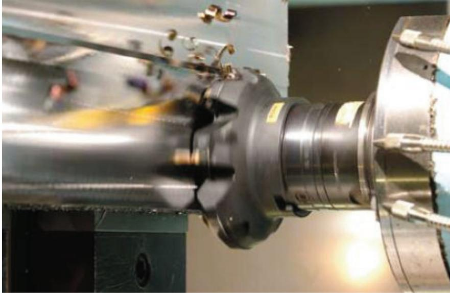
Figure 1.2: Face milling operation [4].
