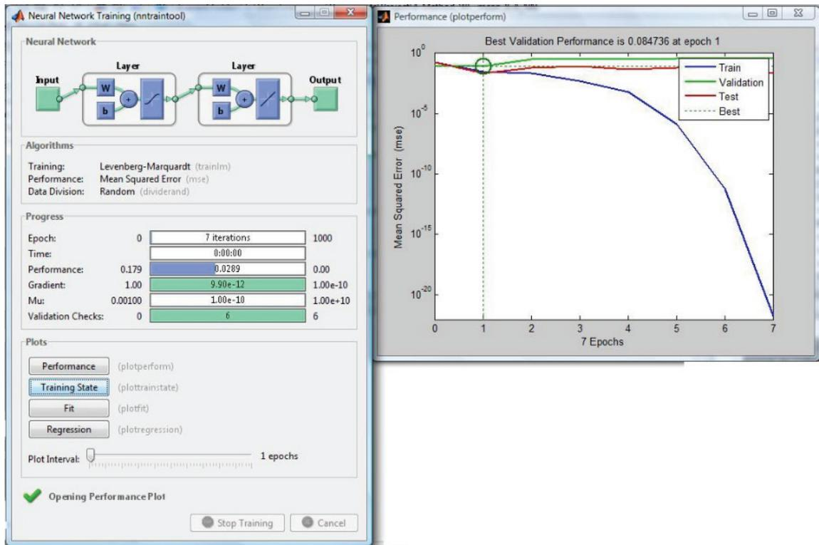
Figure 4.12: The trend of network training with Algorithm 3 for spindle vibration signals.
