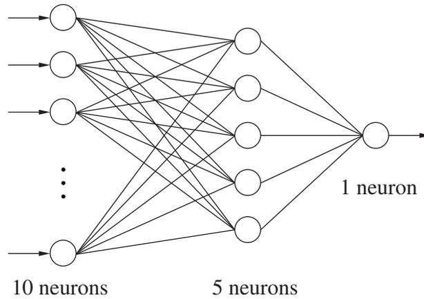
Figure 4.11: The schematic structure of the best network trained with Algorithm 3 for spindle vibration signals.
