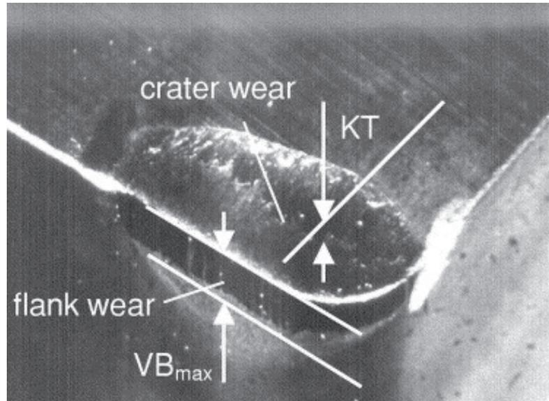
Figure 1.5: Flank and crater wear [13].
