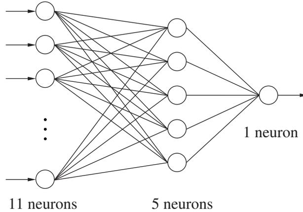
Figure 4.4: The schematic structure of the best network trained with Algorithm 1 for spindle vibration signals.
