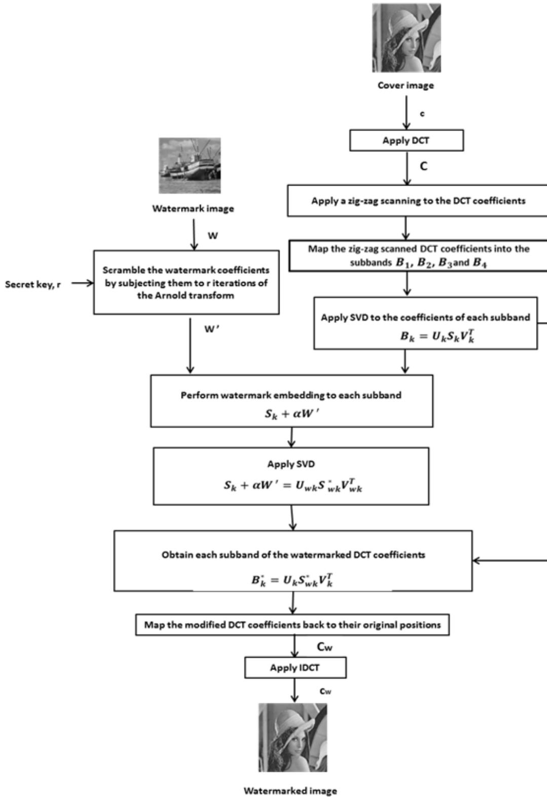
Figure 3.4: Block diagram of the proposed watermark embedding scheme.
