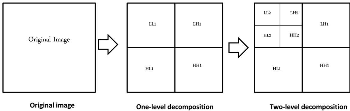
Figure 2.6: Wavelet sub-bands with 2-level decomposition of a 2-dimensional signal.
