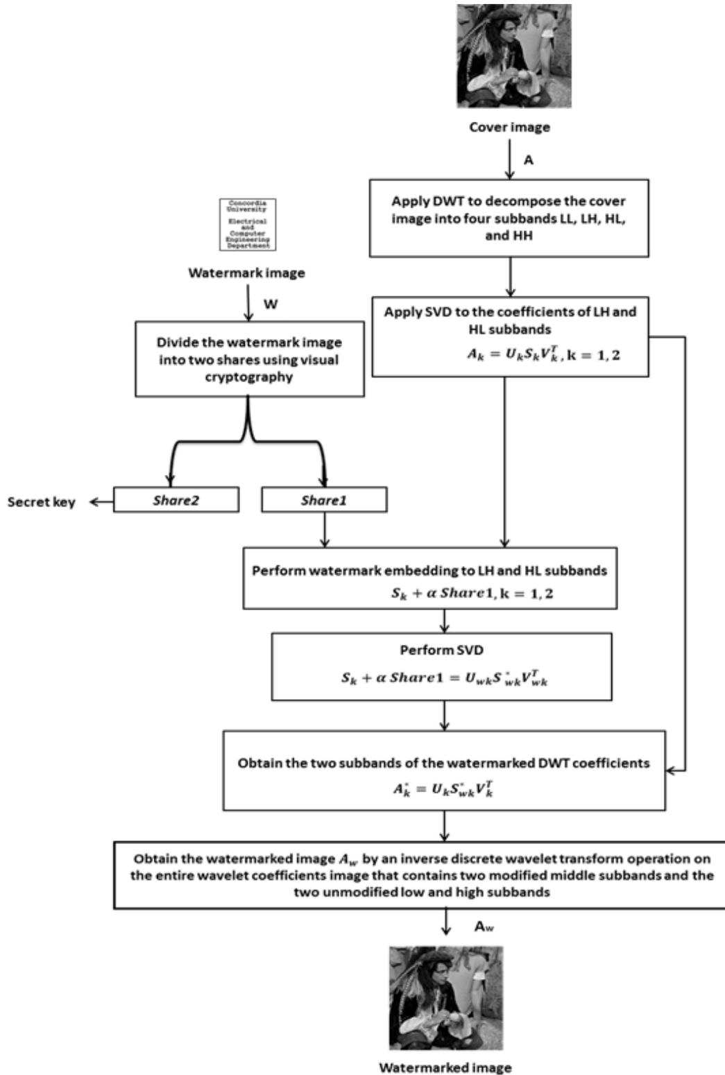
Figure 4.2: Block diagram of the proposed watermark embedding scheme.
