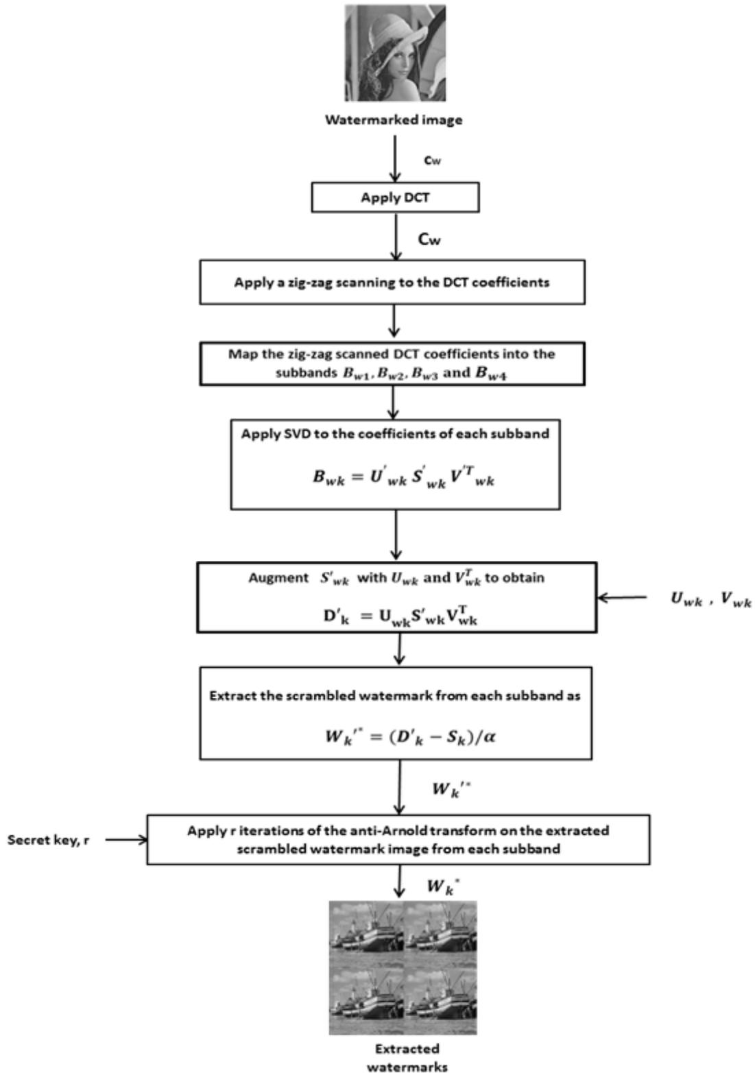
Figure 3.6:Block diagram of the proposed watermark extraction scheme.
