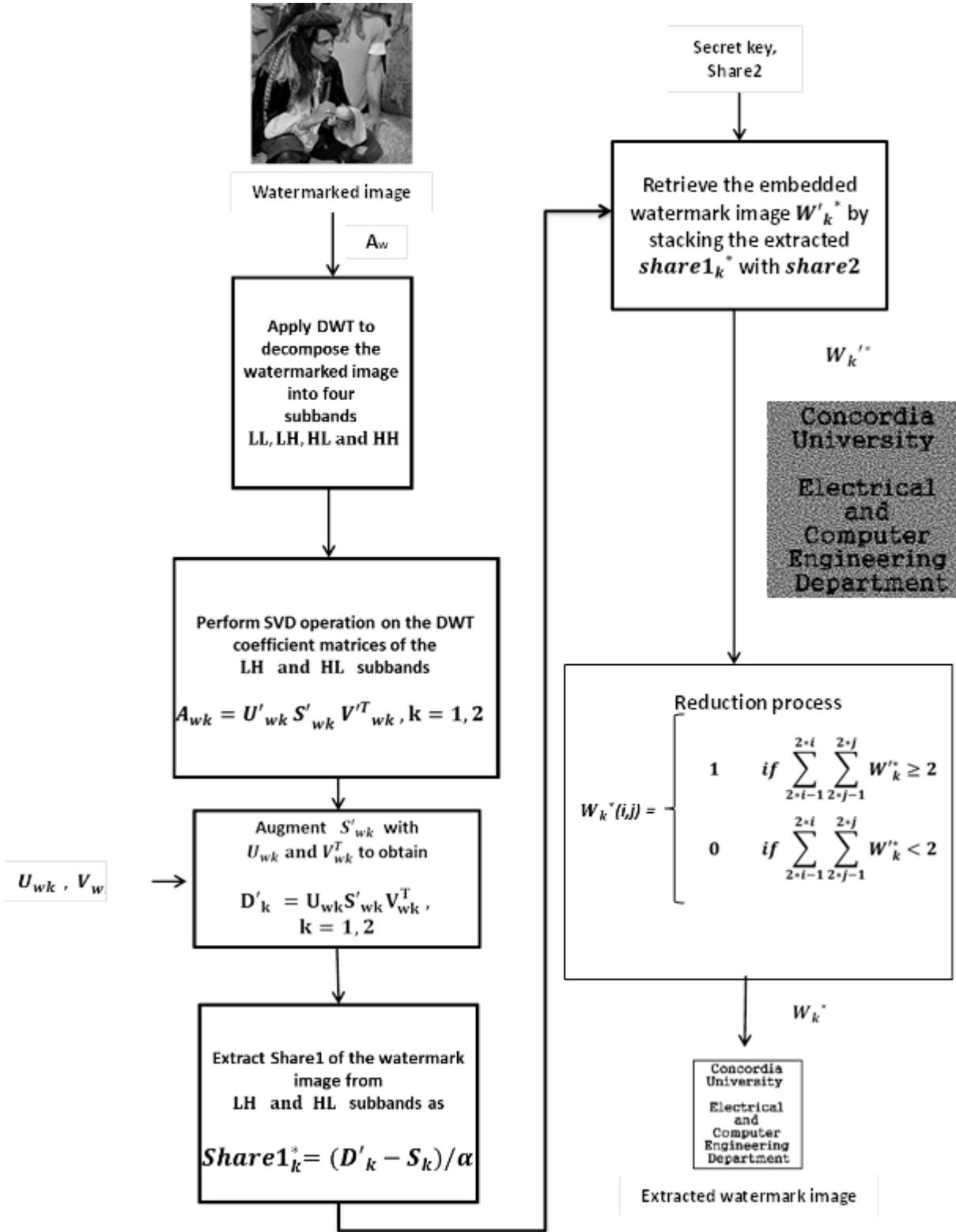
Figure 4.3: Block diagram of the proposed watermark extraction scheme.
