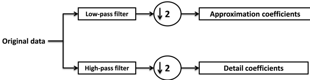
Figure 2.4: Wavelet sub-bands with 1-level decomposition of a 1-dimensional signal.
