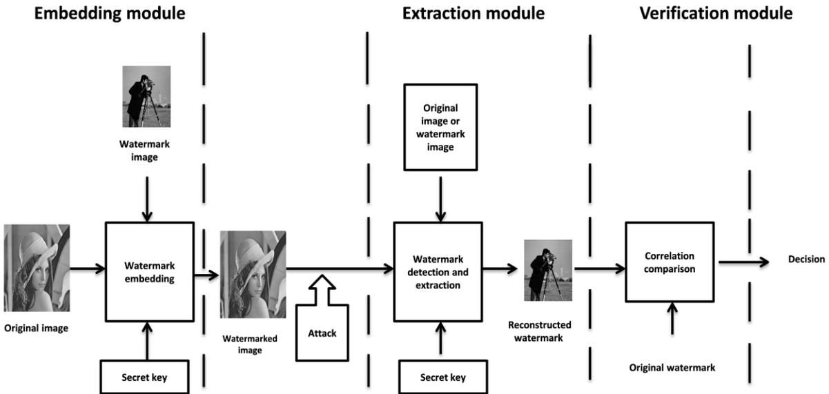
Figure 2.1: A general block diagram for image watermarking.
