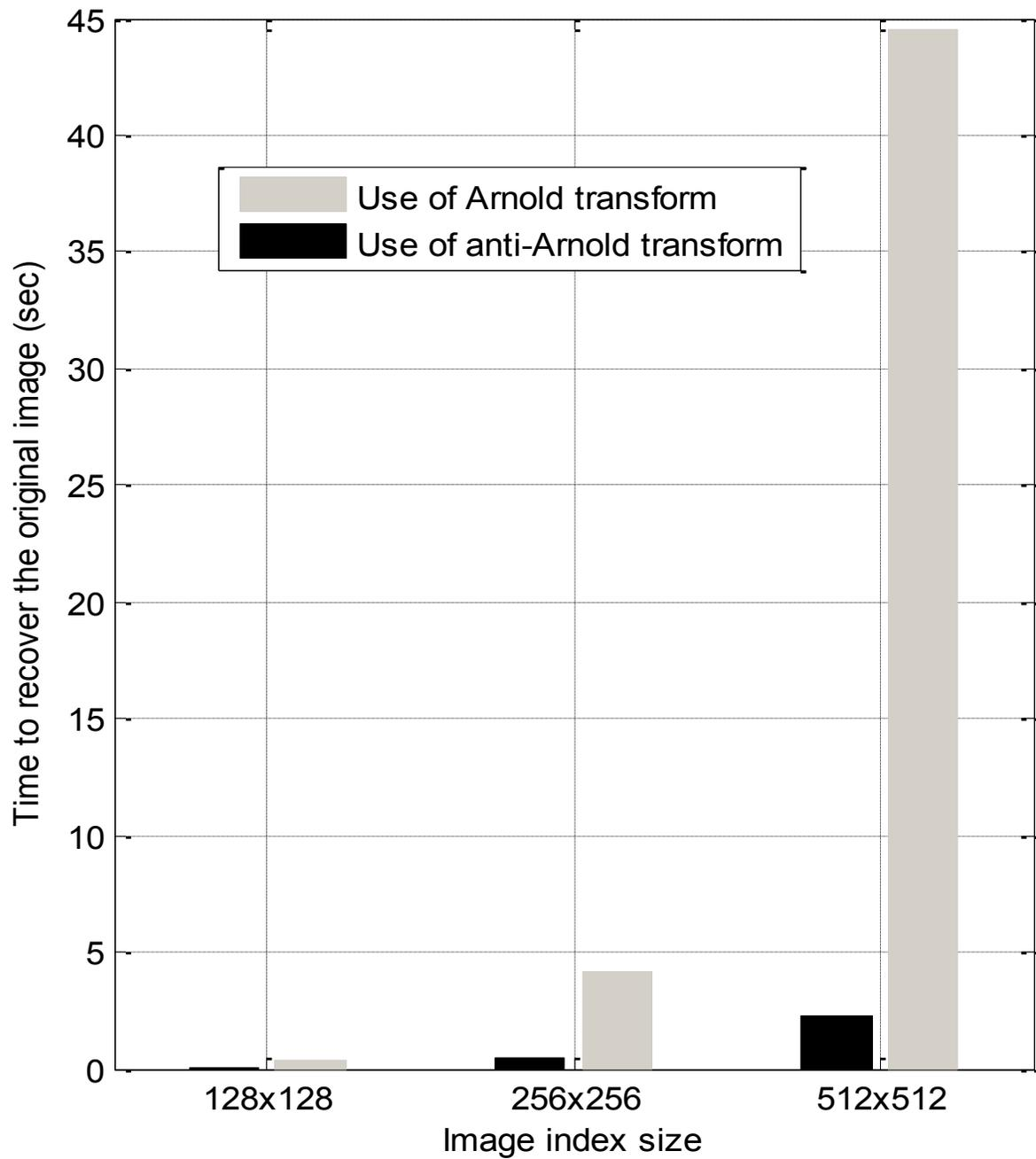
Figure 3.3: Time needed to recover the original image from a scrambled image by using the Arnold and anti-Arnold transforms. The scrambled images have been obtained by applying 20 iterations of the Arnold transform on the original images.
