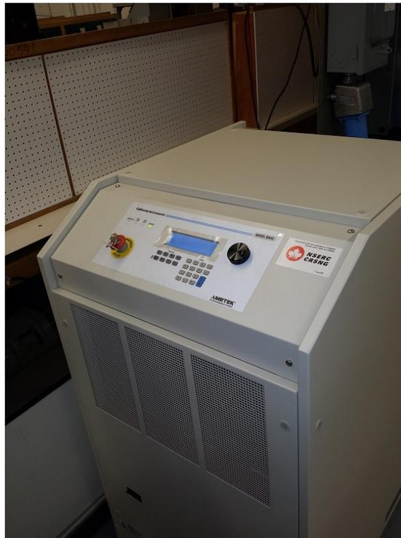
Fig. 3.1. AMETEK® programmable power supply
