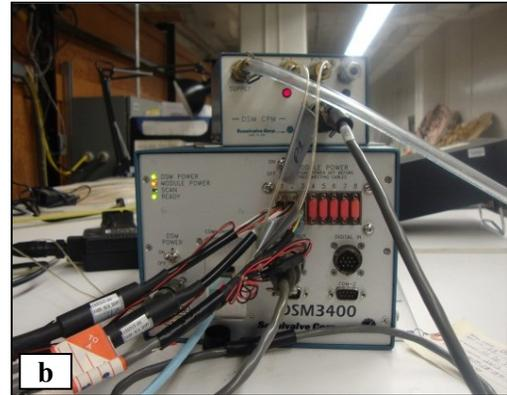
Figure 4.7: Pressure measurement equipment a) Thermal units (T.U. ZOC 64) b) Pressure scan computer (DSM 3400)
