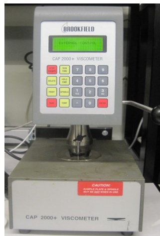
Figure 3.1: Viscometer for measuring dynamic viscosity
