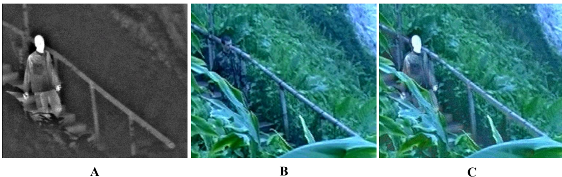
Figure 1.1: Camouflaged target detection: Source images [3]: Thermal image frame (A), Visible image frame (B), Fused image: Thermal-visible fused image (C)
