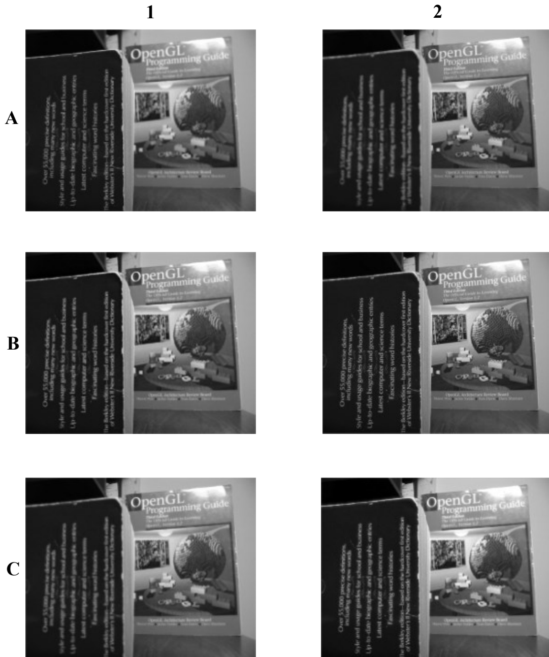
Figure 3.7: Qualitative analysis: Source images Multi-Focus Images (A1 - left focused, A2 - right focused), Fused Results: [7] Laplacian (B1), [2] HOSVD fused (B2), [11] NSCT (C1) , Proposed method (C2) . only if needed
