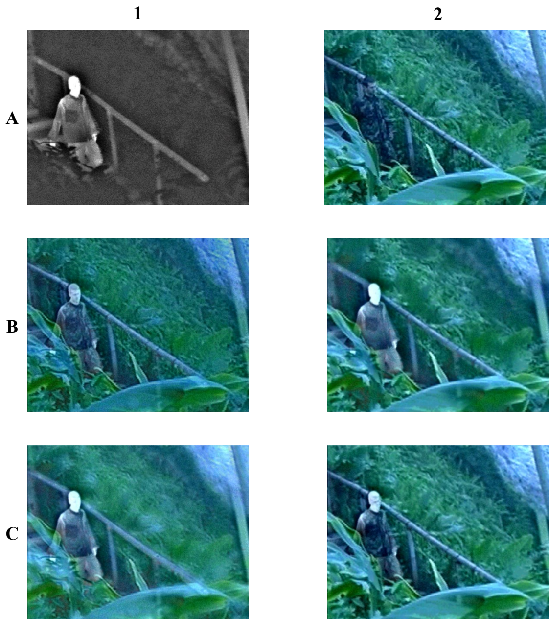
Figure 4.3: Qualitative analysis: Source image [3]: A1 - Thermal, A2 - Visible (frame number: 25), Fused Results: [7] Laplacian (B1), [2] HOSVD fused (B2), [11] NSCT (C1) , Proposed method (C2)
