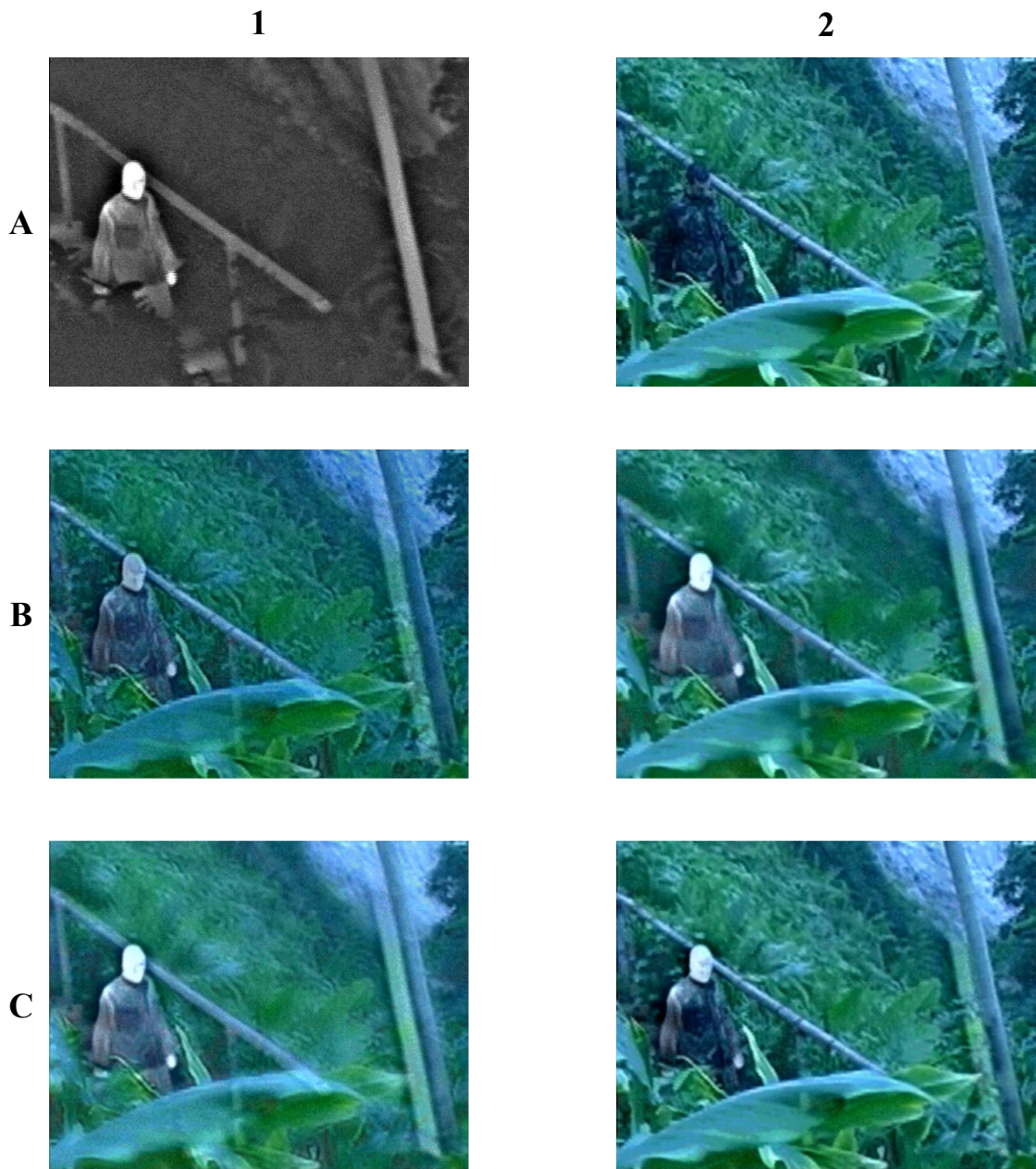
Figure 4.4: Qualitative analysis: Source image [3]: A1 - Thermal, A2 - Visible (frame number: 50), Fused Results: [7] Laplacian (B1), [2] HOSVD fused (B2), [11] NSCT (C1) , Proposed method (C2)
