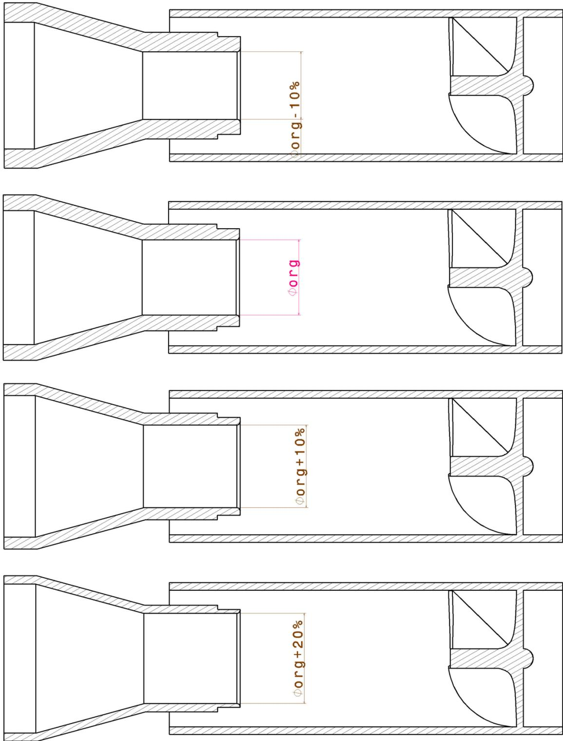
Figure 38- Graphical illustration of diffuser inlet diameter (thickness) variation
