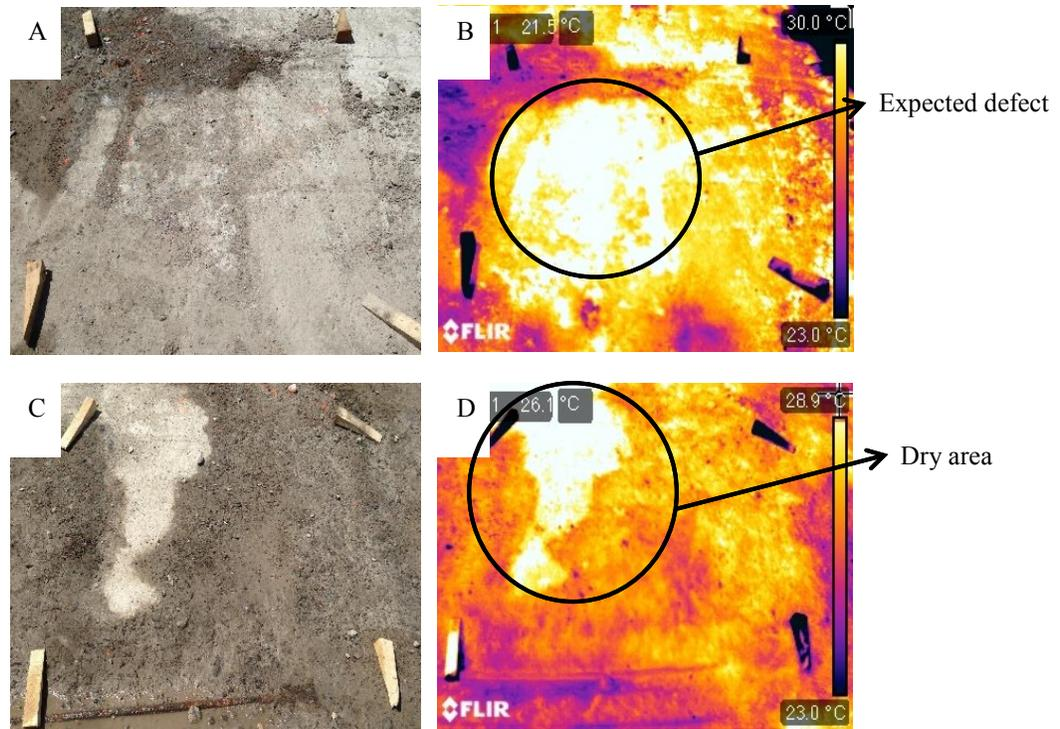
**Figure 4-1 A&B high temperature might refer to a potential defect. C&D high temperature refers to a dry area not a delaminated area**
