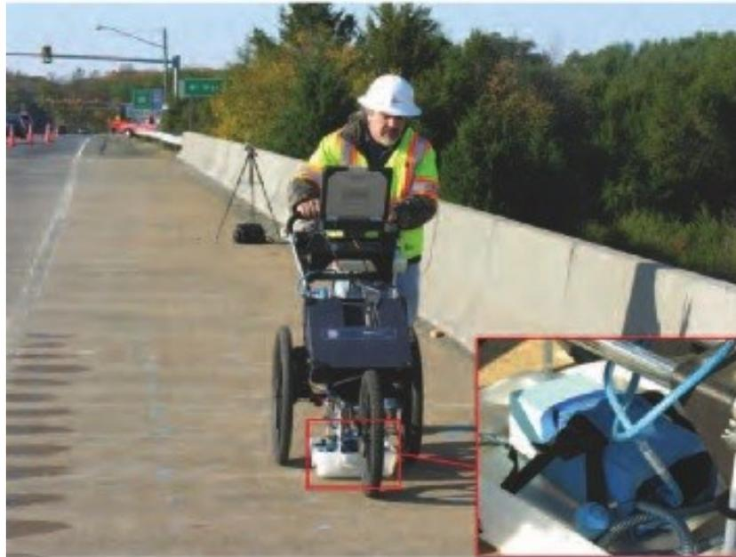
Figure 2-13 GPR unit (Gucunski et al. 2013)
