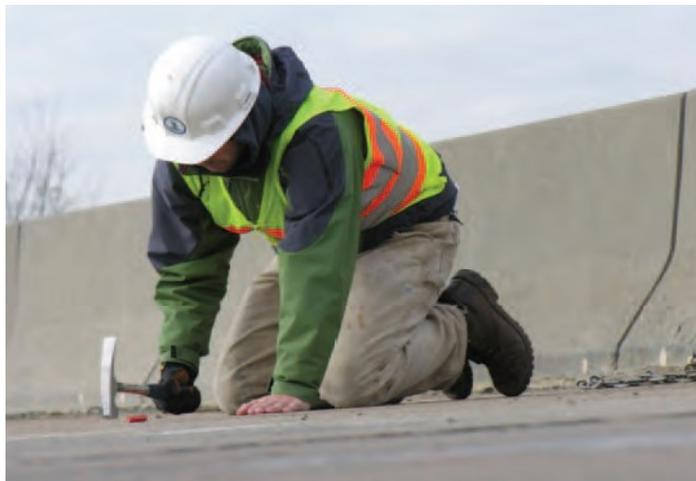
**Figure 2-2 Hammer sounding test (Gucunski et al. 2013)**
