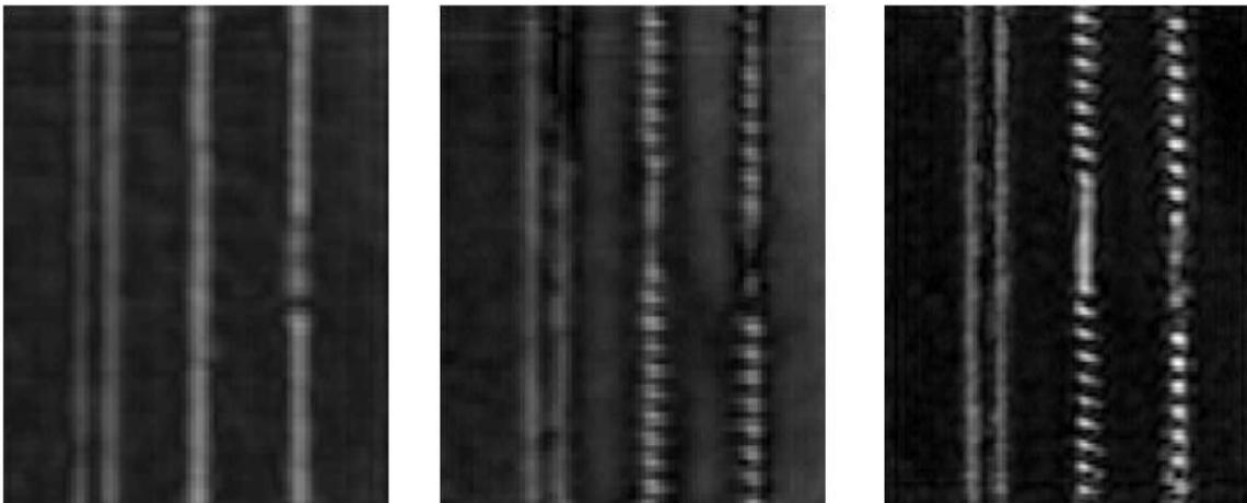
Figure 2-9 SAR detecting reinforcements at different frequencies (Kharkovsky et al. 2011)
