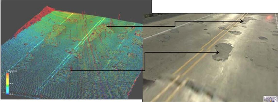
Figure 2-10 A model of a bridge deck using LiDAR (Endsley et al. 2012)
