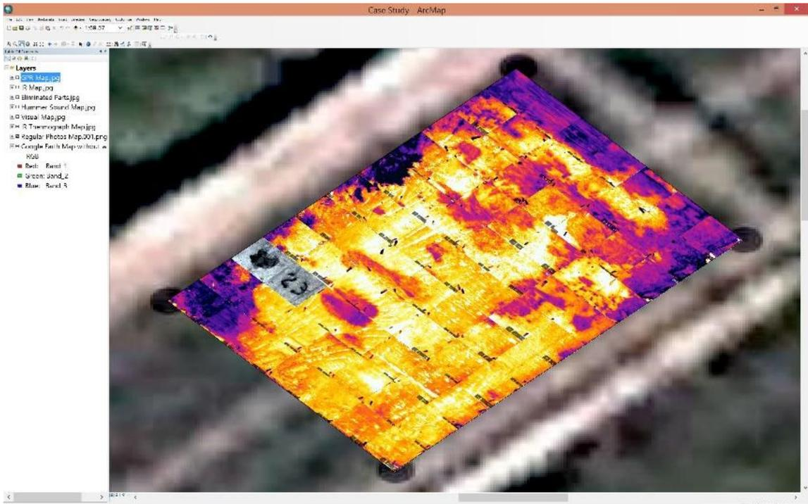
Figure 4-24 ArcGIS snapshot – thermograph map
