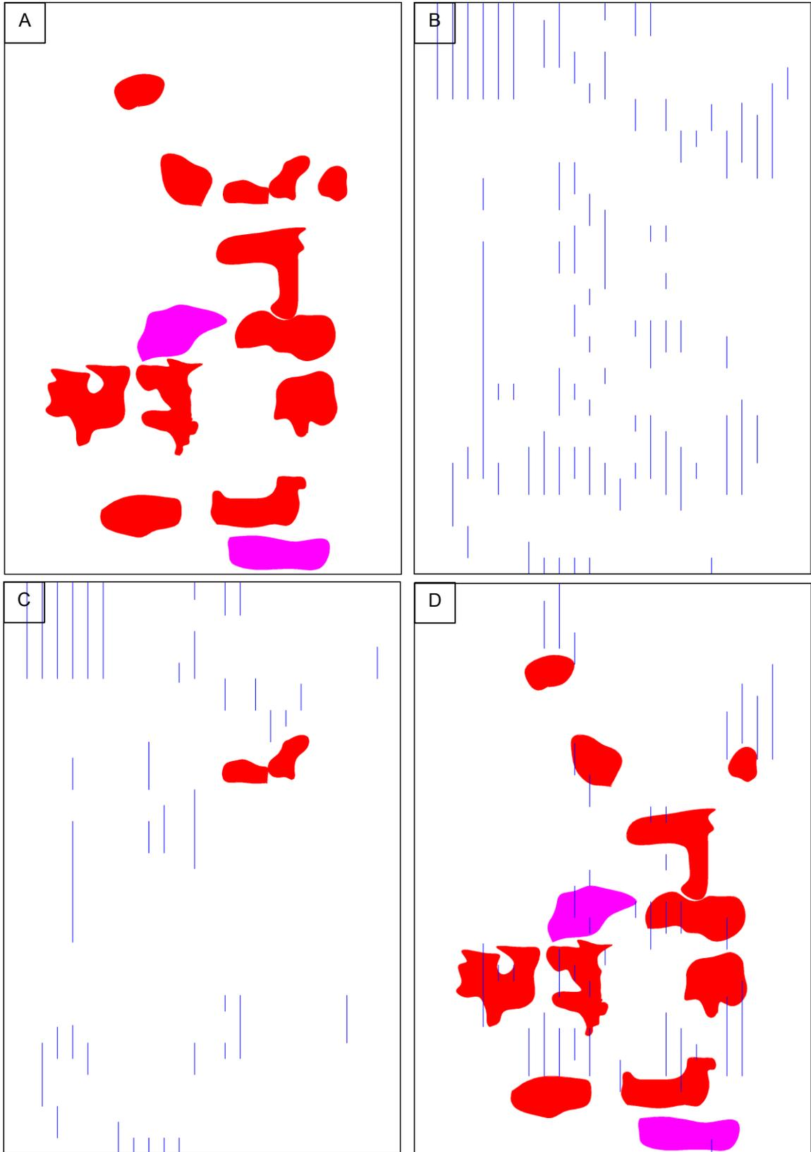
Figure 4-13 Maps of defects A) IR results, B) GPR results, C) Eliminated parts, and D) Hybrid system results
