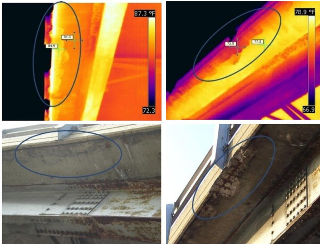
Figure 2-7 IR Detecting subsurface defects (Washer et al. 2010)
