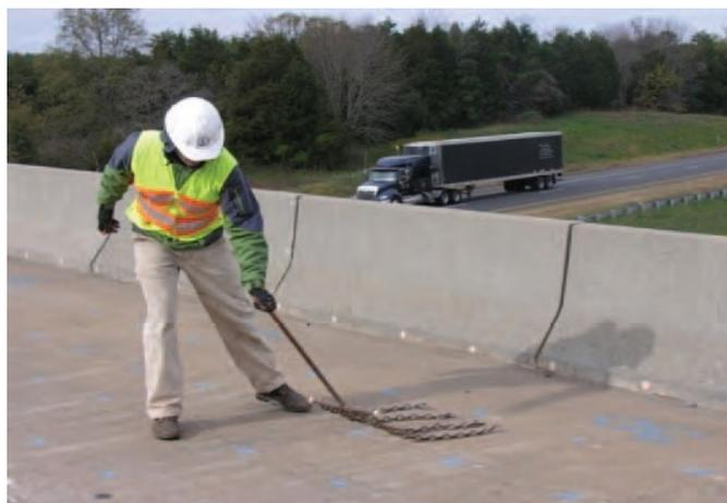
**Figure 2-3 Chain dragging test (Gucunski et al. 2013)**
