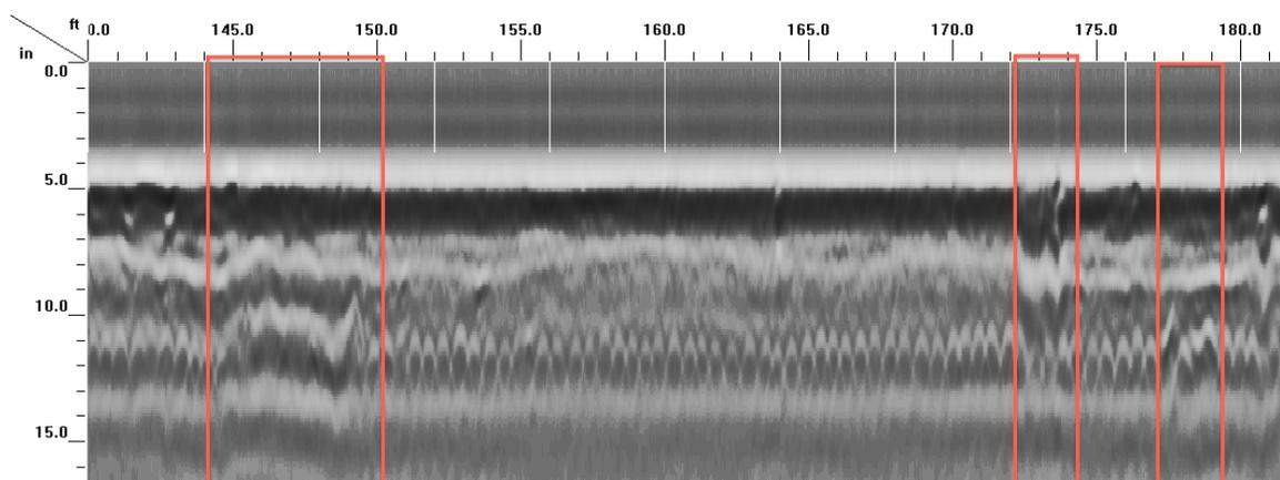
Figure 4-3 GPR scan and potential delamination
