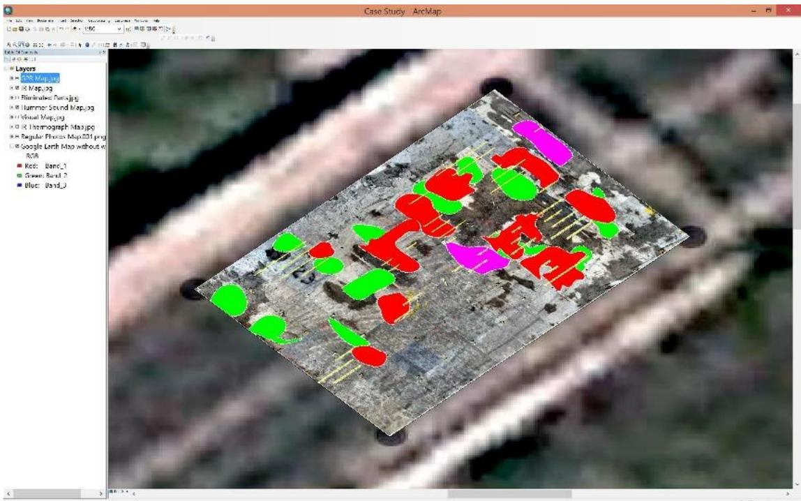
Figure 4-21 ArcGIS snapshot – hybrid system and hammer sound test
