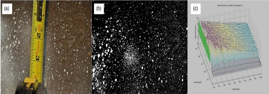
Figure 2-12 Using DIC in finding the displacement response of an I-Beam (Vaghefi et al. 2011).
