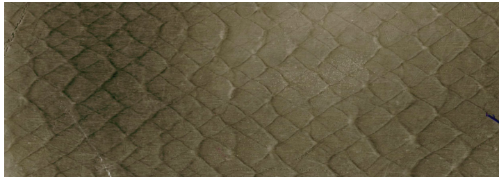
Figure 1.1 A smoked foil showing the characteristic fish scale in C_2H_2 + 2.5 O_2 + 70\%Ar at P_o = 12 kPa.
