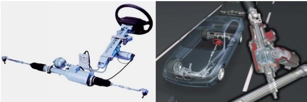
Figure 1.2: Designs of steering mechanisms for implementations of AFS control: (a) a steer-by-wire (SBW); and (b) a mechanical planetary gear system [44].
