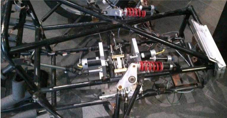
Figure B.3: Designed AIFS prototype installed on a project vehicle structure.
