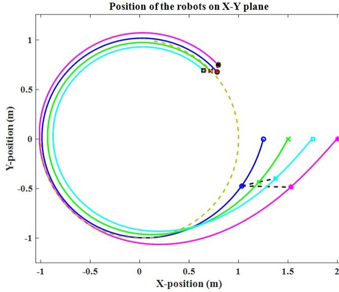
Figure 11: Formation control trajectories of four robots.
