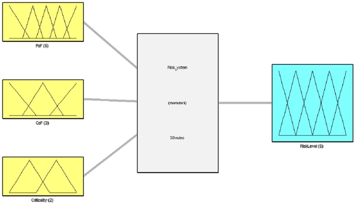
**Figure 5.12 Risk Index Model Configuration on MATLAB**
