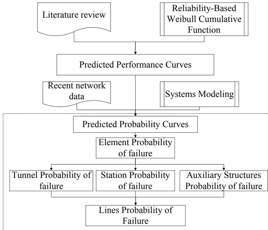
**Figure 3.3 Probability of Failure Sub-Model Outline**
