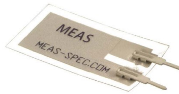
Fig. 2.1. LDT0-028K laminated PVDF polymer thin film [35]
