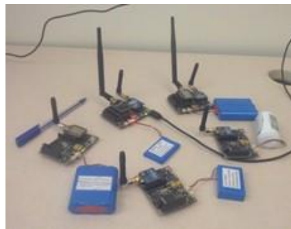
Figure 4-15: Wasp mote platform mobile nodes
