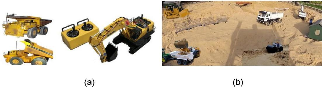
Figure 4-46: SA-GPS Prototype Mounted on Scaled Equipment
