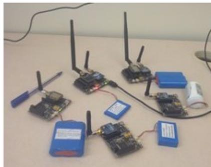
Figure 4-15: Wasp mote platform mobile nodes
