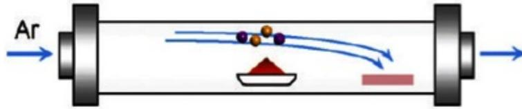
Figure 2.2.1: Argon transport gas flows  $\text{Bi}_2\text{Se}_3$  vapour down the quartz tube towards target substrate. Figure from *Mlack* [23]
