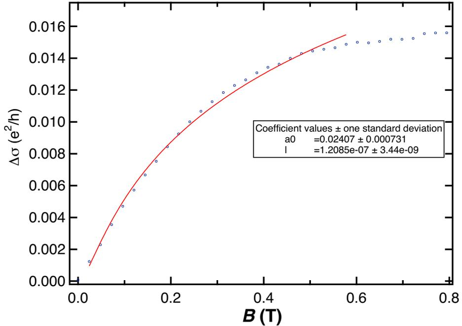
Figure 4.2.3: Fitting the HLN model to the data of sample D, we extract a value of  $\alpha=0.024$
