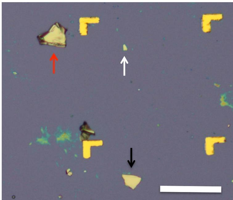
Figure 2.3.1: Preliminary characterization of mechanically exfoliated flakes using an optical microscope
