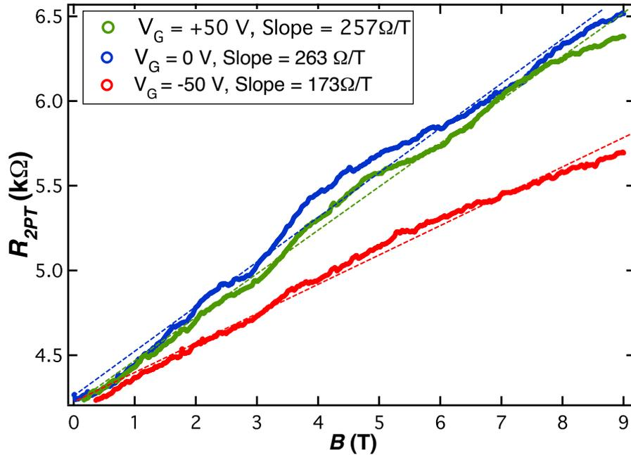
Figure 4.1.6: Resistance vs magnetic field for different gate voltages. The slope of linear fits: (+50V):  $257 \text{ } \Omega/T$ , (0V):  $263 \text{ } \Omega/T$ , (-50V):  $173 \text{ } \Omega/T$
