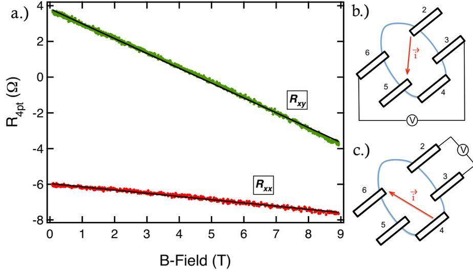
Figure 4.1.4: a.) The 4-probe Hall measurement shows partial mixing of transverse and longitudinal modes due to contact geometry: b.) Transverse Hall signal ( $\rho_{xy}$ , Green line) c.) Longitudinal Hall signal ( $\rho_{xx}$ , Red line)
