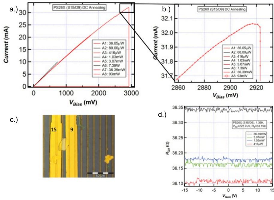
Figure 5.2.3: Joule Heating in suspended sample E: a.) Repeatedly ramping up the current b.) Current saturation leading to device failure c.) Optical image of suspended sample d.) Gatesweeps show resistance is converging with annealing
