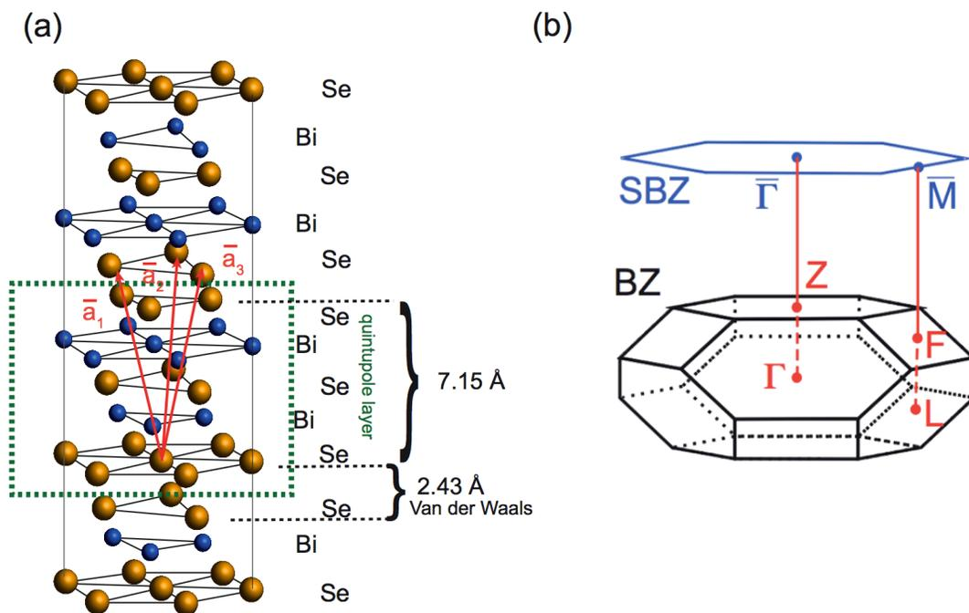
Figure 3.1.1: (a) The lattice structure and (b) the bulk and surface Brillouin zones of crystal  $\text{Bi}_2\text{Se}_3$  Figure from *Bianchi* [26]
