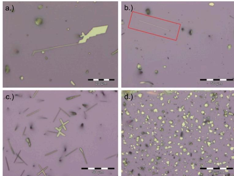
Figure 2.2.2: Vapor-Solid growth from powderized  $\text{Bi}_2\text{Se}_3$  a.) Interesting step-like growth results in a nanoribbon attached to a planar crystal with many corners b.)  $50\ \mu\text{m}$  long nanoribbon c.) X-shaped crystals d.) Triangular and hexagonal stacked nano plates.
