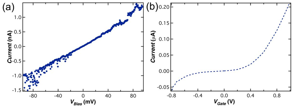
Figure 3.1.4: (a) A 2-point bias sweep reveals a large resistance  $R = 74\ \text{M}\Omega$ , and shows disorder, (b) With constant source/drain voltage, the gate voltage is swept over  $\pm 1\ \text{V}$ . A breakdown of the  $\text{SiO}_2$  substrate leads to the backgate making a current connection directly to the gold electrodes
