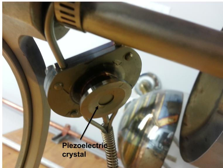
Figure 2.4.6: The resonance frequency of the crystal thickness monitor is measured by a RF circuit, and is sensitive to nanometer thick metal layers
