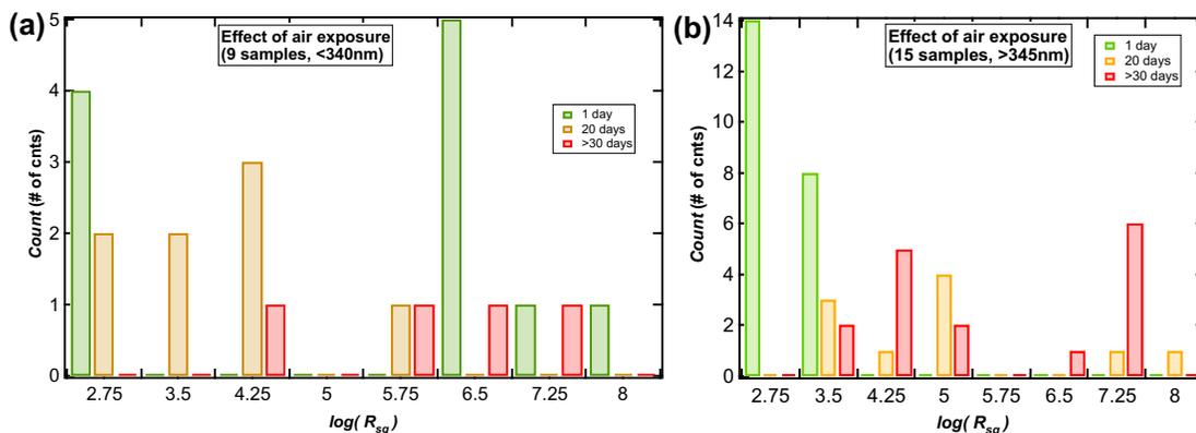
Figure 3.3.4: Contact resistance vs air exposure time: (a) For thin samples, minimizing exposure to air is insufficient to create low resistance contacts. (b) In thicker samples the contact resistance is reduced by minimizing air exposure
