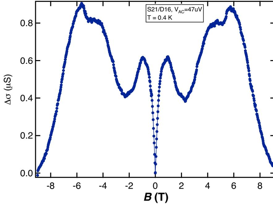
Figure 4.1.7: A clear low B-field peak is observed along with subsequent large oscillations at increasing field strength
