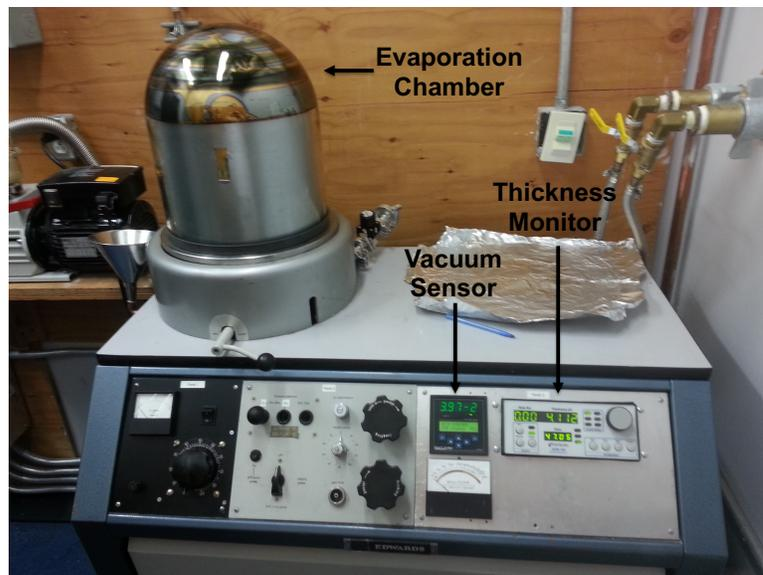
Figure 2.4.4: Metal deposition of the contacts is done using a diffusion pumped thermal evaporator
