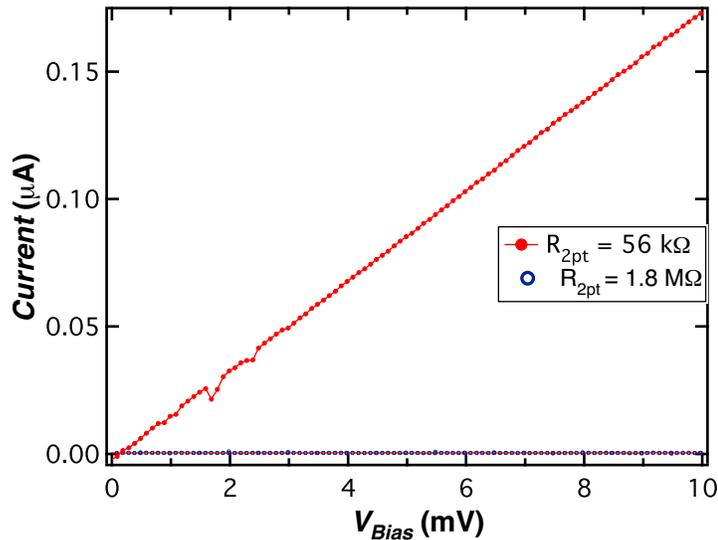
Figure 3.1.5:  $I - V$  plot shows a linear source/drain dependence. 2pt resistance is extracted from the slope
