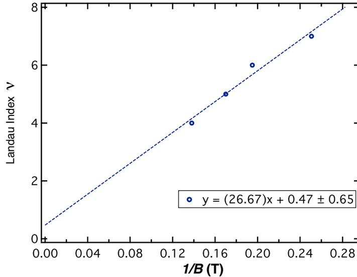
Figure 4.3.2: Landau fan diagram for sample C ( $t = 38$  nm,  $T = 1.5$  K) shows the filling fraction assignment vs  $1/\text{magnetic field}$
