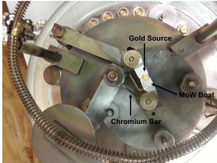
Figure 2.4.5: Current is passed through either a Chromium bar or a Gold nugget, creating metal vapour under vacuum
