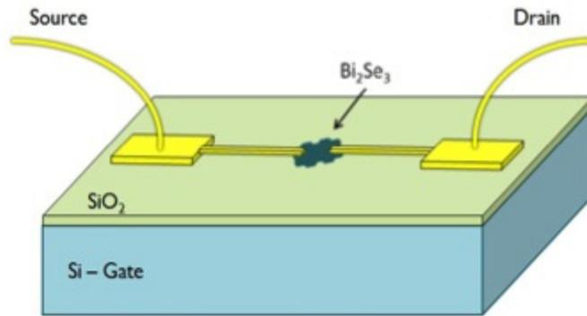
Figure 2.4.1: Source and drain electrodes physically contact the  $\text{Bi}_2\text{Se}_3$  crystal, while the gate is capacitively coupled via the  $\text{SiO}_2$  dielectric film.
