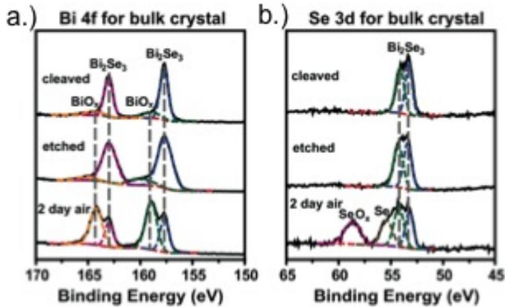
Figure 3.2.2: (a) Bi and (b) Se XPS Spectra for  $\text{Bi}_2\text{Se}_3$  shows the formation of an oxide layer over 2 days, with both Bi and Se binding to Oxygen in the air. Samples etched with an Argon plasma (middle panel) display a reduction in the level of oxidation [7]
