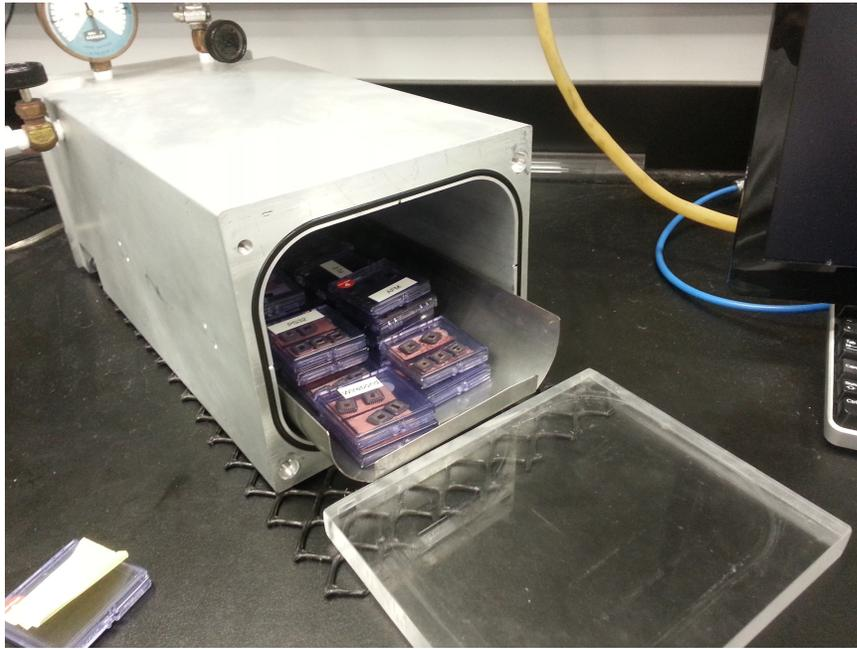
Figure 2.4.8: Prepared samples are stored under vacuum to minimize exposure to air
