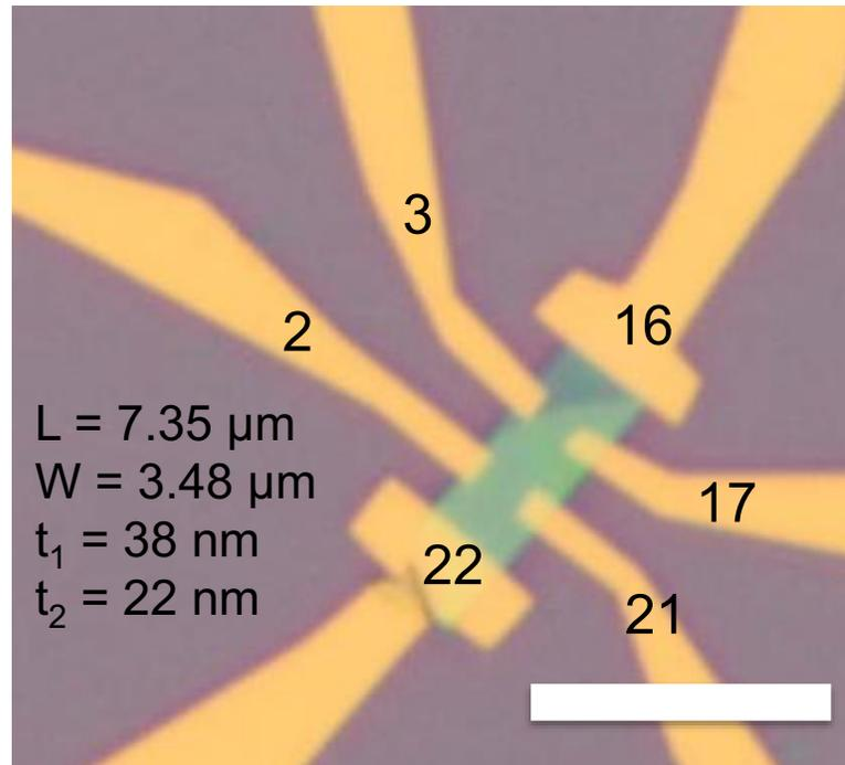
Figure 5.1.1: Mechanically exfoliated  $\text{Bi}_2\text{Se}_3$  of  $22 \text{ nm}$  with lithographically defined Gold electrodes. Scale bar is  $10 \mu\text{m}$ .
