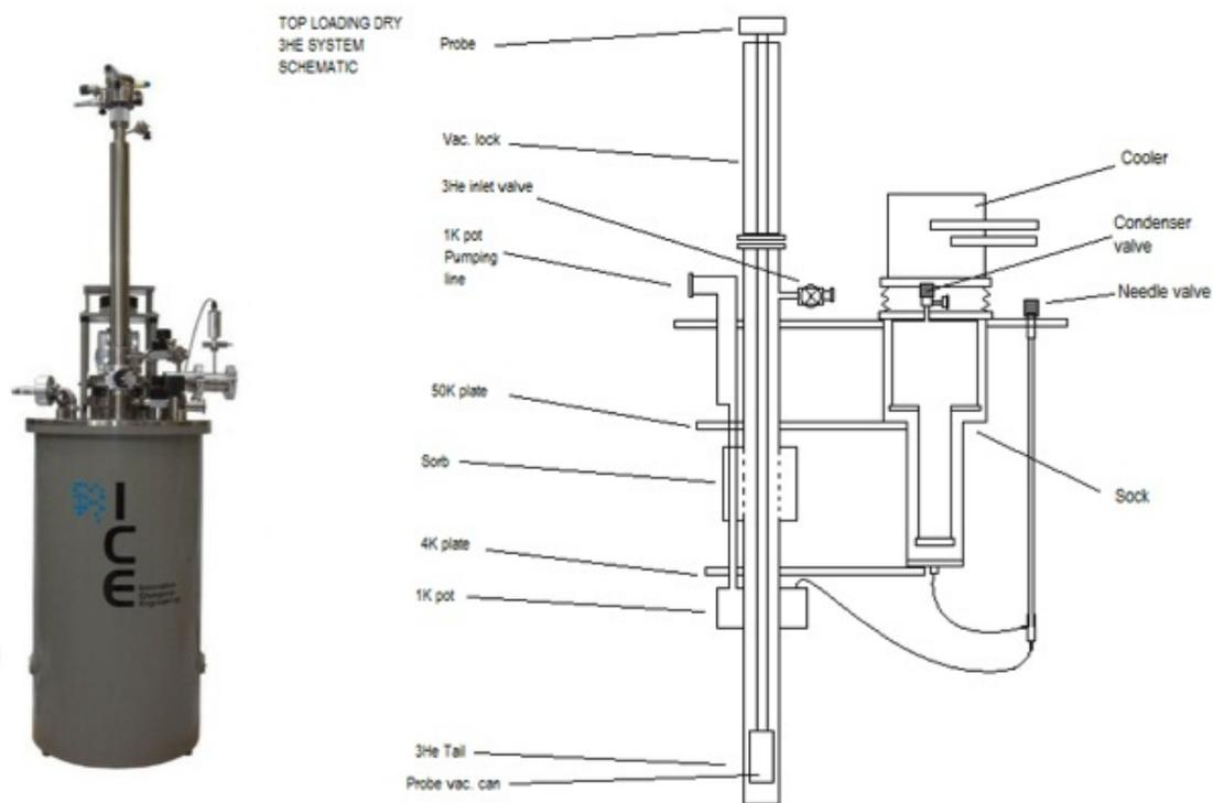
Figure 2.5.2: 0.3 K fridge: The LHe-3 cryostat has an inner sample space buffered by a LHe-4 pot held at 1.2 K. The needle valve allows controlling the flow of LHe-4
