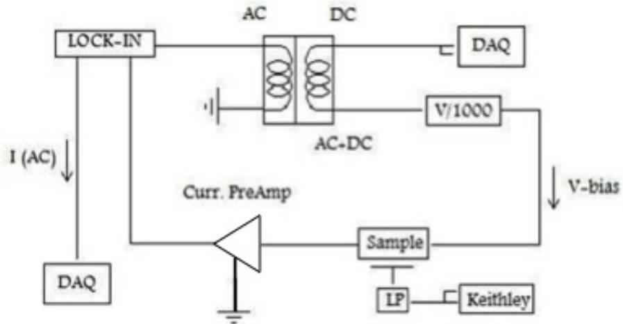
Figure 2.5.3: Our AC circuit uses a transformer to add an AC perturbation atop a DC source signal
