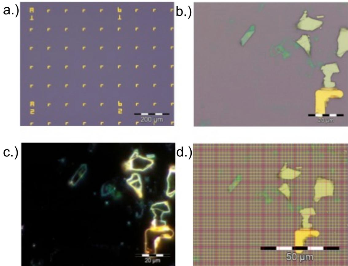
Figure 2.4.2: a.) Prepatterned Gold reference grid for flake location b.) Bi<sub>2</sub>Se<sub>3</sub> flakes are exfoliated onto the grid c.) Dark field imaging shows surface and edge uniformity, suggesting the crystalline nature of the flake d.) Optical image overlaid with a digital coordinate system for CAD design of EBL electrodes
