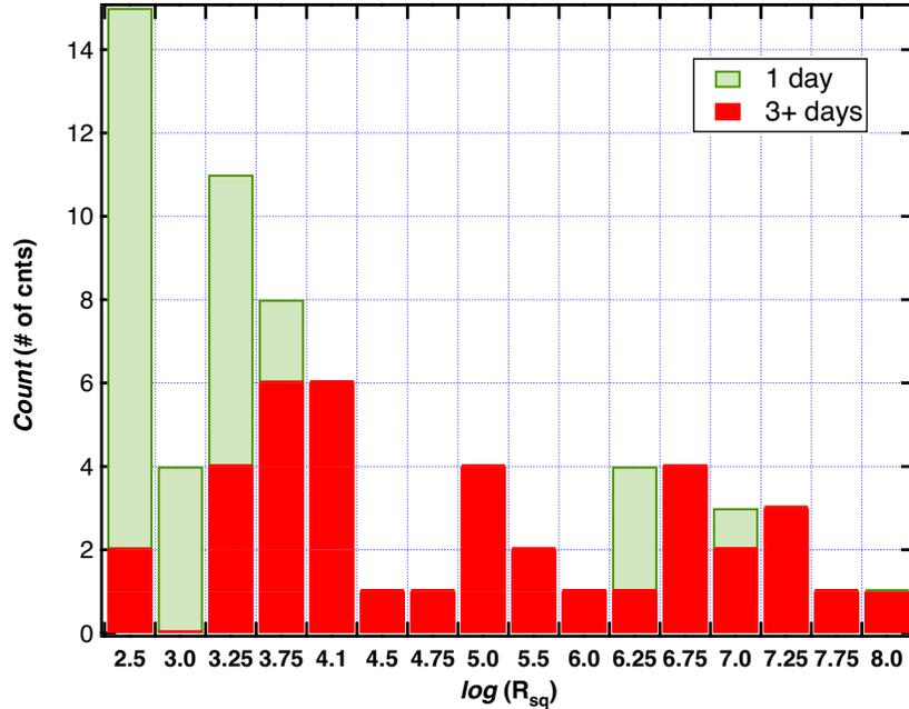
Figure 3.2.5: Histogram showing the number of low resistance contacts is increased by limiting the time of air exposure to 1 day
