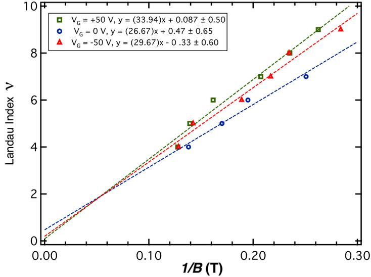
Figure 5.1.2: Landau fan diagram showing the filling fraction assignment vs  $1/B$ , for sample C with thickness 38 nm, at  $T = 1.5 \text{ K}$
