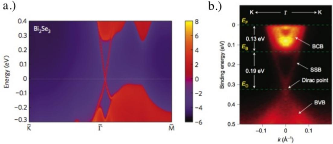
Figure 3.1.2: The band structure of crystal  $\text{Bi}_2\text{Se}_3$ : a.) Theoretically calculated local density of states [9], and b.) The bandstructure experimentally observed via ARPES [8]
