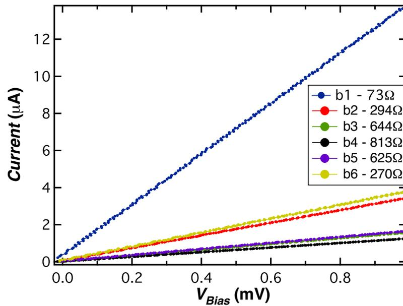
Figure 3.2.4: Current-Bias curves show a significantly lower resistance compared to sample G
