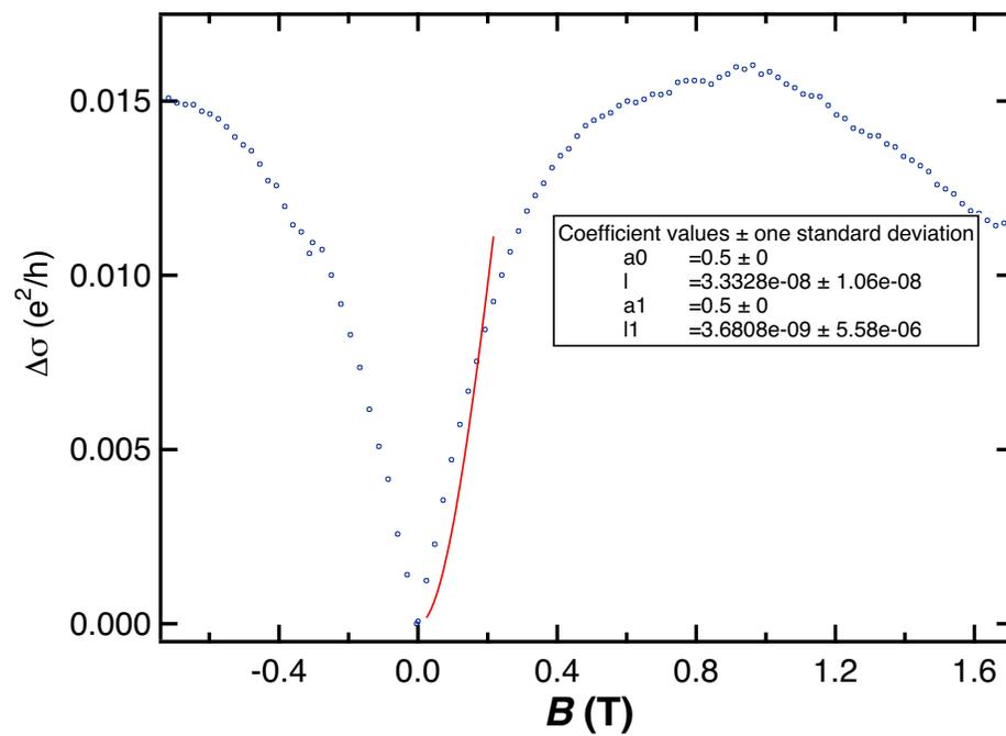
Figure 4.2.4: Fixing  $\alpha = 0.5$  we find the HLN model does not fit the data, suggesting the low-field peak is not due to WAL
