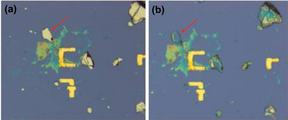
Figure 3.2.1: (a) Freshly exfoliated  $\text{Bi}_2\text{Se}_3$  crystal flakes, (b) Left in open air for 3 months, the crystals are severely degraded
