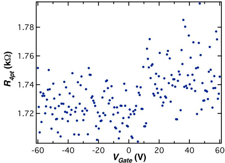
Figure 3.1.6: With a constant source/drain voltage applied, the 4-point resistance does not show gate dependence
