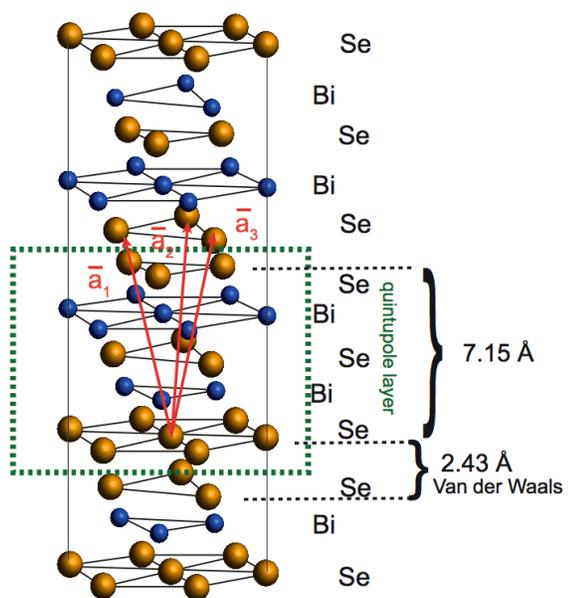
Figure 1.1.3: The crystal structure of bismuth selenide is made of planar trigonal lattices, bonded together 5 layer stacks at a time. Figure taken from *Bianchi et al.* [26]
