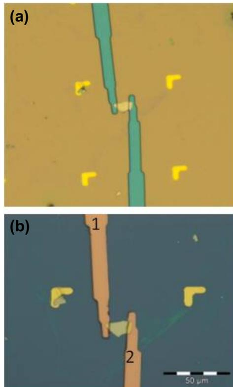
Figure 3.3.2: (a) After defining electrode positions using photolithography, a plasma etch is done to clean the exposed area of  $\text{Bi}_2\text{Se}_3$  under the contacts (b) Metal electrodes are evaporated and the photoresist is lifted off, resulting in a sample with gold contacts on the surface
