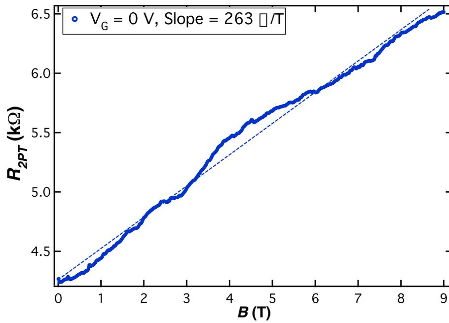
Figure 1.2.1: Resistance vs magnetic field in sample C shows small oscillations on top of a linear slope, indicating parallel bulk and surface transport
