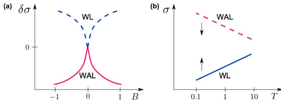
Figure 4.2.2: a.) Weak localization and anti-localization display opposing peaks near zero magnetic field b.) Both WAL and WL display a linear magnetoresistance at higher fields [19]
