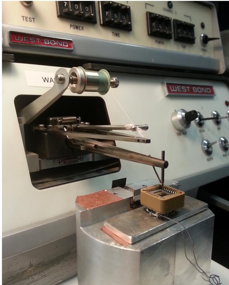
Figure 2.4.7: Device packaging: our wire bonder scales down the users movements in order to precisely attach 25 micron thick Aluminum wires using an ultrasonic pulse
