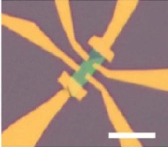
Figure 2.4.3: Bi<sub>2</sub>Se<sub>3</sub> flake with Hall bar geometry after metal electrode evaporation (scale bar is 10  $\mu\text{m}$ )
