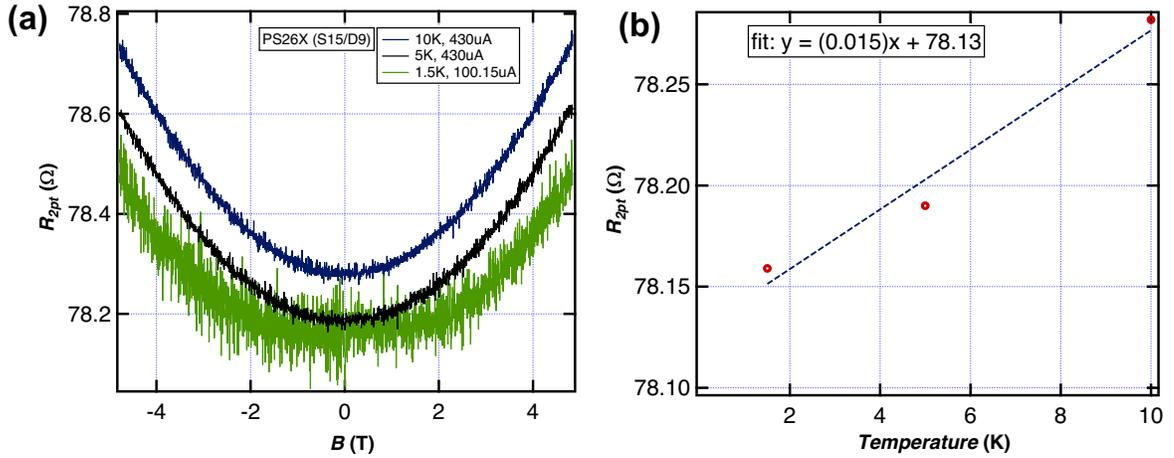
Figure 5.2.2: (a) Magnetic-field dependence of sample E at  $T = 1.5, 5, 10$  K, (b) The 2-point resistance at  $B = 0$  Tesla
