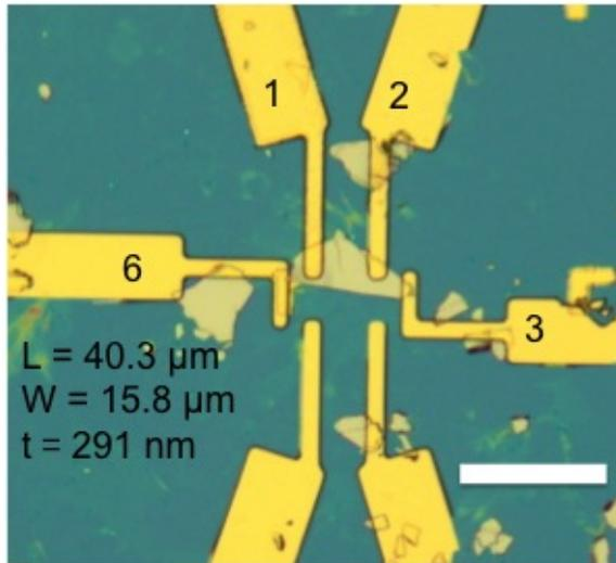
Figure 3.2.3: 4-point sample B, fabricated with moderate air exposure (20 days)
