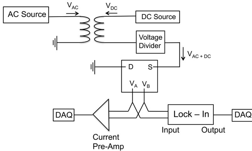
Figure 4.1.2: 4-pt surface adds an AC signal atop a DC bias. Voltage is sent to the sample via the source (S) electrode, and sent to ground by the drain (D). Voltage
