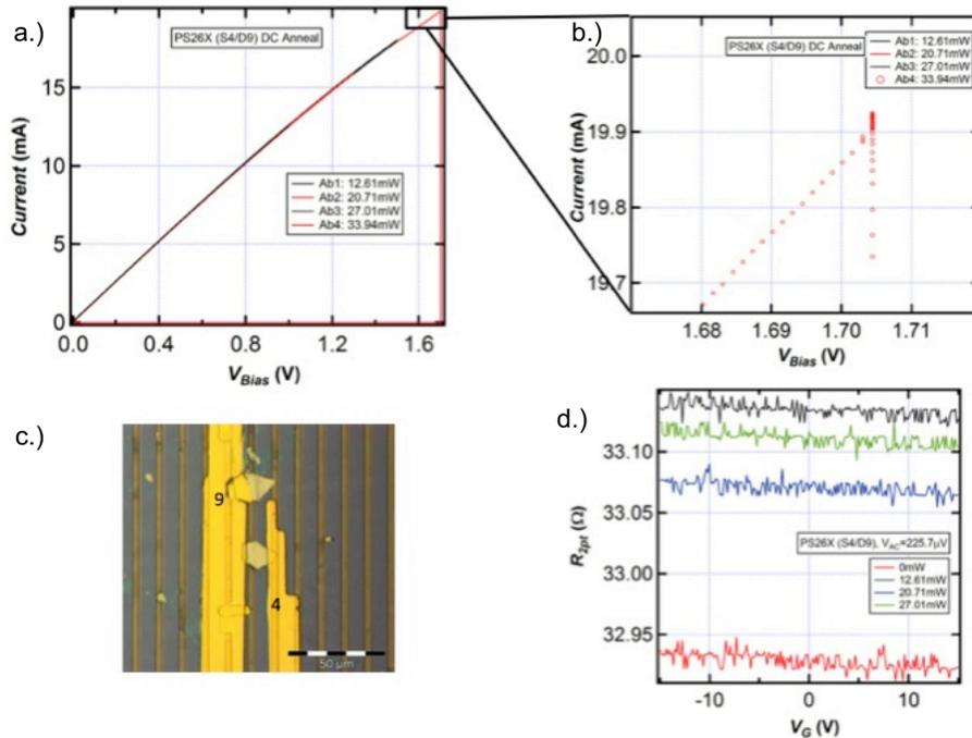
Figure 5.2.4: Joule Heating in suspended sample F: a.) Repeatedly ramping up the current b.) Current saturation leading to device failure c.) Optical image of suspended sample d.) Gatesweeps show resistance is converging with annealing
