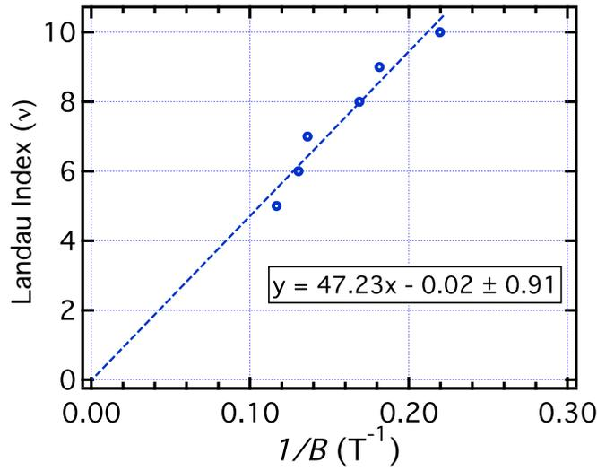
Figure 4.3.5: Replotting the fan diagram using both  $R_{xx}$  and  $R_{xy}$  to locate oscillations, we find an intercept of 0, however with an error of  $\pm 0.91$  we cannot conclude about the Berry's Phase
