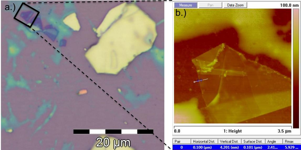
Figure 2.3.2: Thin flake characterization: a.) Optical and b.) Atomic Force Microscope images of a 6 nm-thick exfoliated  $\text{Bi}_2\text{Se}_3$  flake
