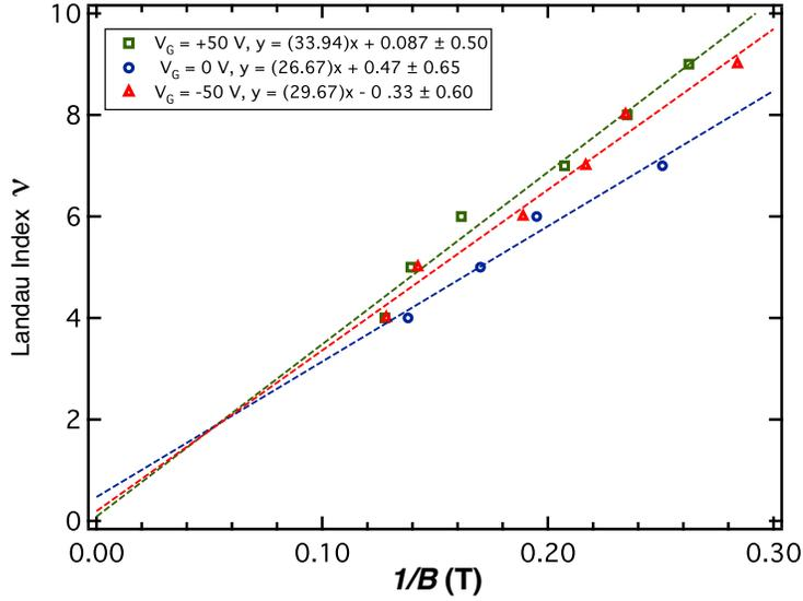
Figure 4.3.3: Landau fan diagram shows the change in carrier density with electric field
