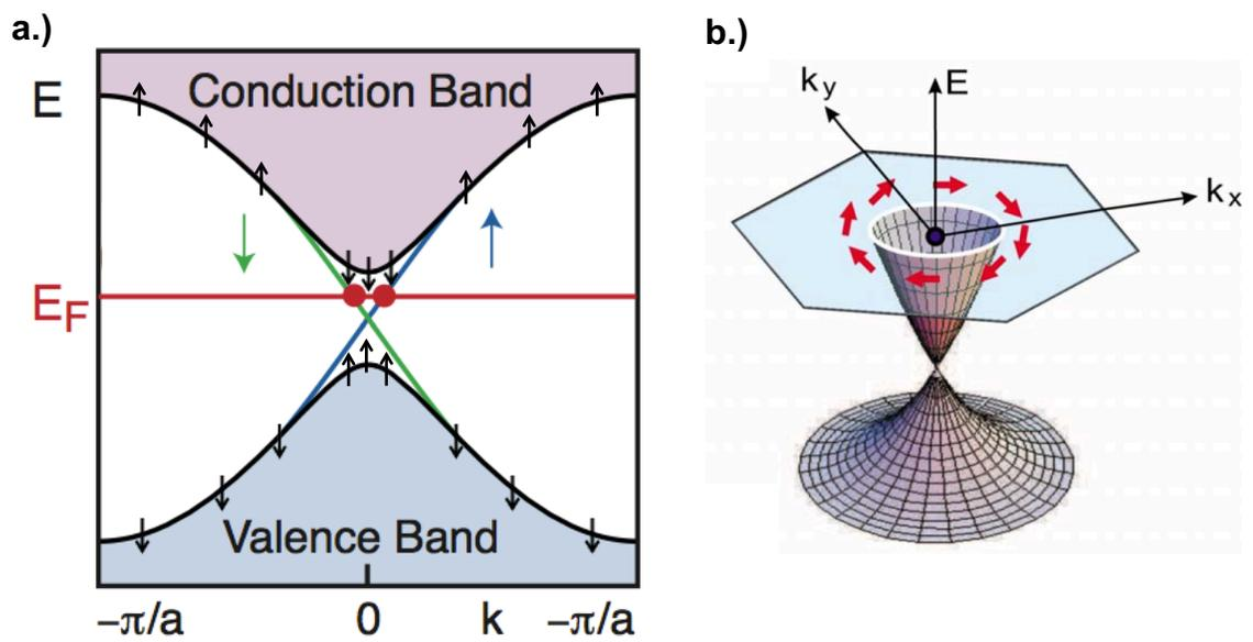
Figure 1.1.2: Band Structure of a topological insulator. (a) Band inversion results in topologically protected surface states in a bulk bandgap (green and blue lines). Figure adapted from *Hasan* et al. [28] (b) Spin-momentum locking on a topological surface state. Figure from *Hsieh* [3].
