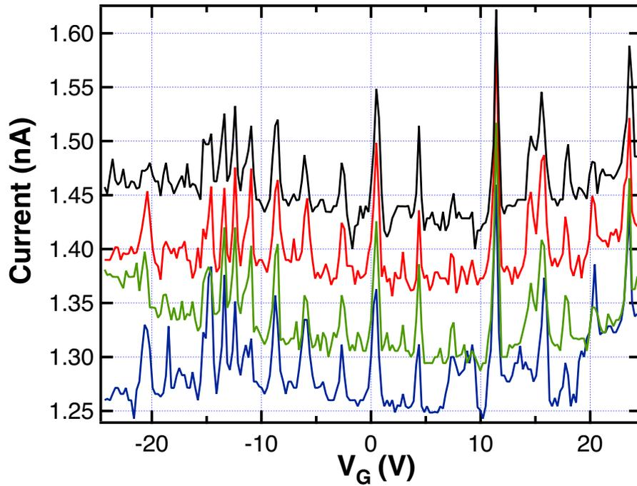
Figure 4.4.1: Current peaks in  $V_{Gate}$ : Robust spikes in current in gatesweeps at constant magnetic field ( $B = 0, 5, 6, 7$  Tesla). The change in current over 50 V change in gate voltage is roughly 5%
