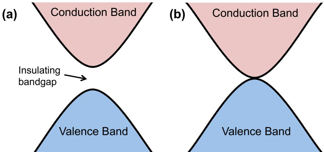
Figure 1.1.1: Band structure in solids: (a) A trivial insulator with  $Z_0$  topology has a large insulating energy gap where no conduction occurs, (b) When the valence and conduction bands meet, a  $Z_1$  crossing occurs resulting in metallic conduction states
