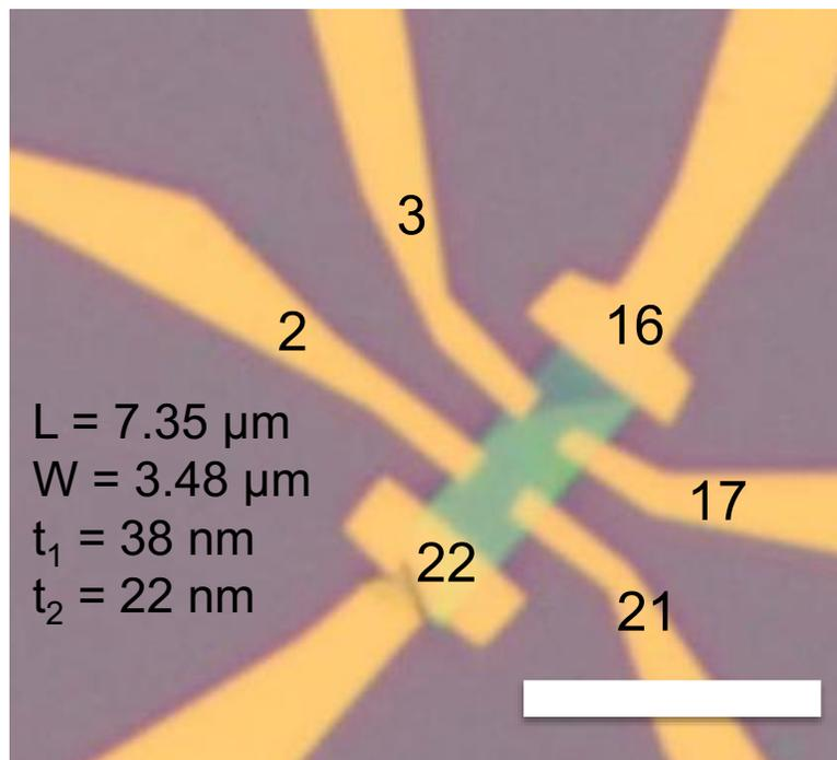
Figure 1.2.2: Mechanically exfoliated  $\text{Bi}_2\text{Se}_3$  of 22 nm with lithographically defined Gold electrodes. Scale bar is 10  $\mu\text{m}$ .
