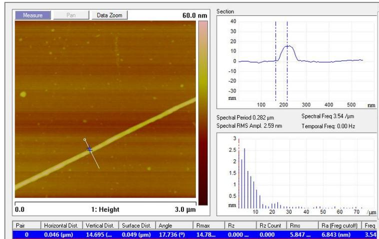
Figure 2.2.3: AFM measurement of a 15 nm thick ribbon with uniform edges
