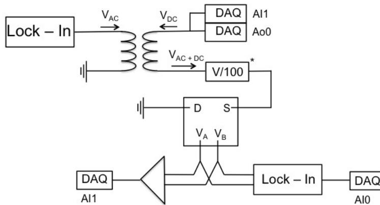
Figure 2.5.4: The 4-pt AC circuit uses a transformer to add an AC perturbation atop a DC source signal and measure the DC bias separately from the AC contribution
