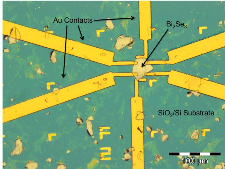
Figure 2.0.1: Photolithographically defined electrodes on a Bi<sub>2</sub>Se<sub>3</sub> crystal with a Hall bar geometry
