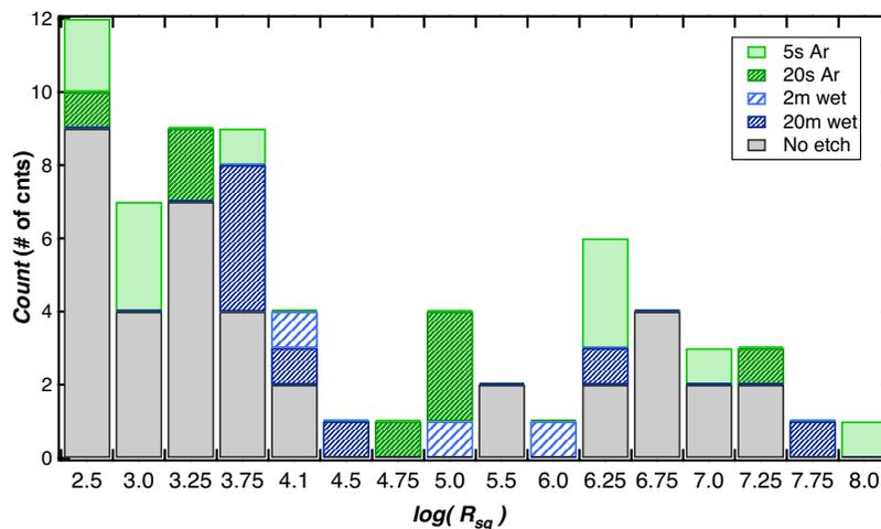
Figure 3.3.3: Number of contacts vs  $\log(R_{sq})$  for many devices whose contacts were made with 5s and 20s long Ar RIE etches, 2m and 20m TCE cleaning and without any additional contact cleaning
