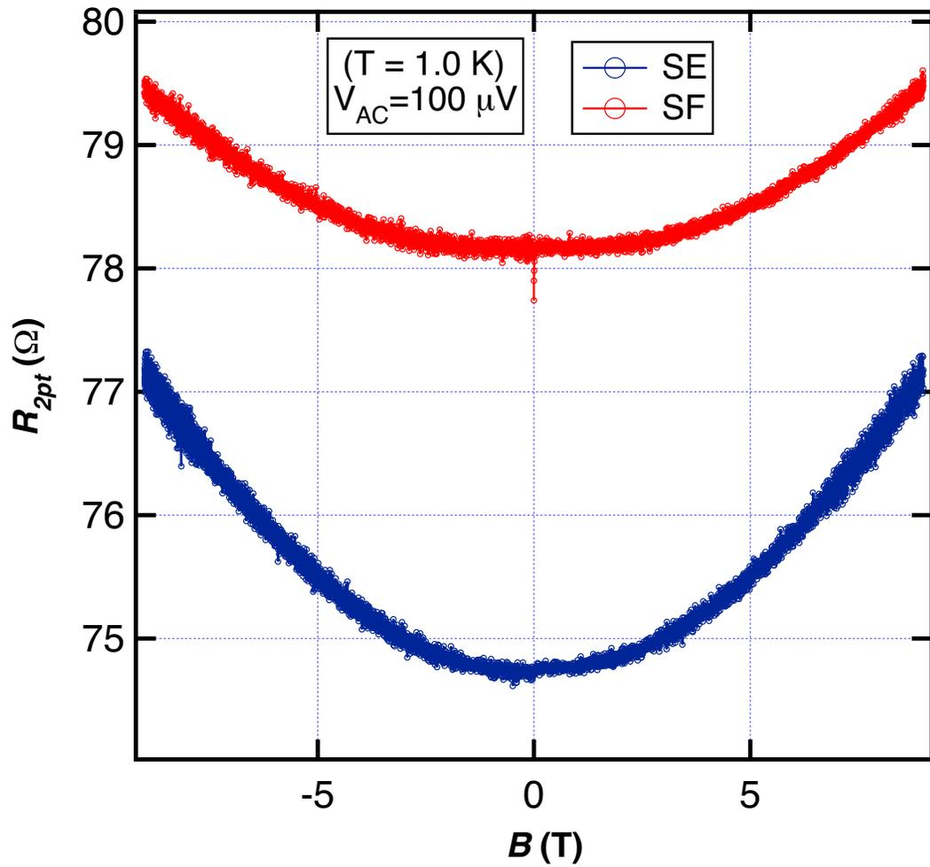
Figure 5.2.1: Magnetic-field dependence of suspended topological insulator transistors E and F at  $T = 1$  K
