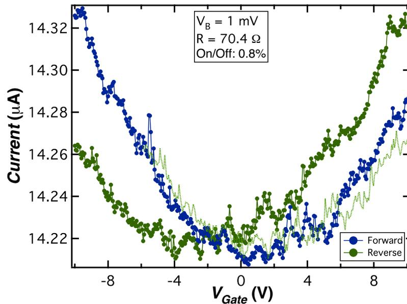
Figure 3.4.1: Current versus back gate voltage graph in a low contact resistance sample
