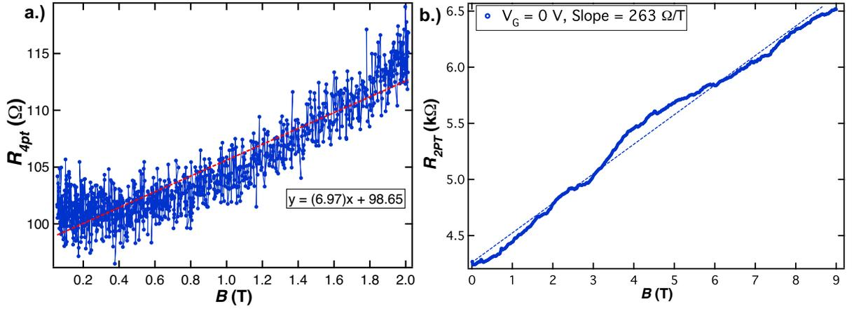
Figure 4.1.5: R vs B: a.) The 4-point measurement in sample B shows a partial mixing of  $R_{xx}$  and  $R_{xy}$  at low-fields b.) The 2-point measurement in sample C displays oscillations on top of a linear slope.
