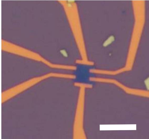
Figure 3.1.3: Ultrathin  $\text{Bi}_2\text{Se}_3$  crystal with EBL defined contacts (Scale bar =  $10\ \mu\text{m}$ )
