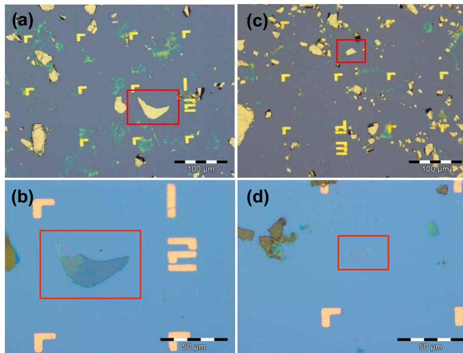
Figure 3.3.1: Non selective Argon plasma etches the surface of  $\text{Bi}_2\text{Se}_3$  crystals: (a) An opaque flake of a higher thickness is reduced to the point of becoming translucent, shown in (b). The smaller flake in panel (c) is reduced to effectively nothing in (d)
