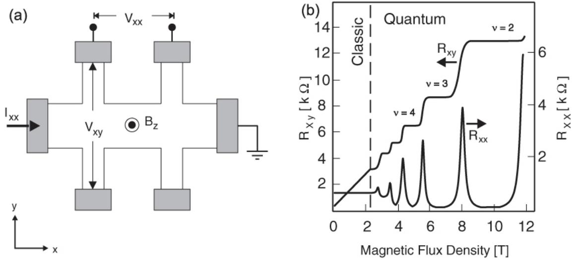
Figure 4.1.3: a.) 6-point Hall Bar geometry b.) Longitudinal and transverse Hall resistance. Figure from Janssen et al. [35]
