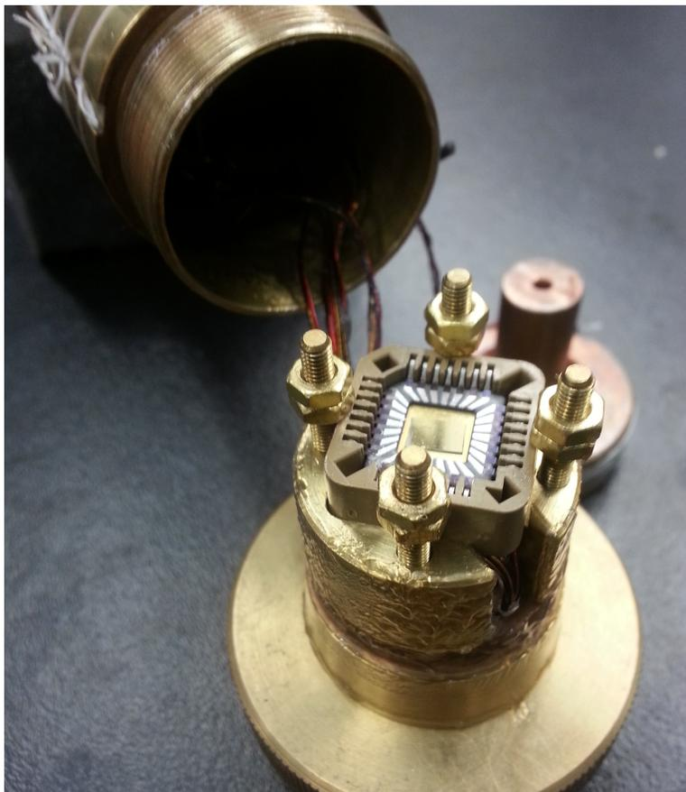
Figure 2.5.1: Sample testing: A packaged sample, loaded in the measurement probe of our  $^3\text{He}$  cryostat
