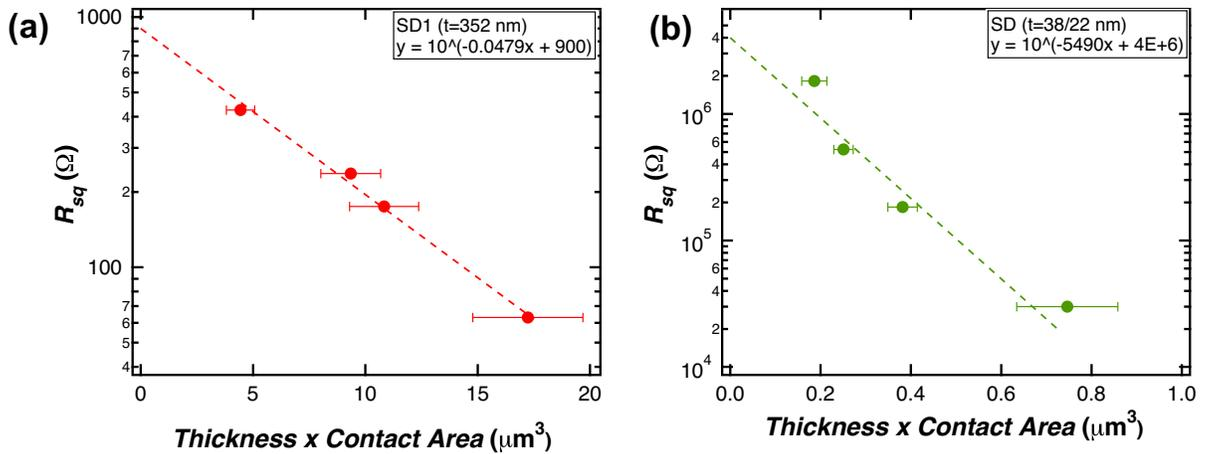
Figure 3.2.6: In two samples of thickness (a)  $t = 352$  nm and (b)  $t = 38$  nm, 22 nm, the contact resistance per unit area scales logarithmically with the volume of the contact, defined by contact area times sample thickness.
