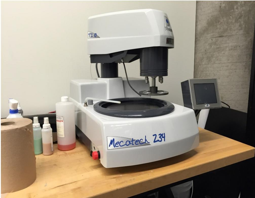
**Figure 4.26 Mecatech 234 polishing machine**
