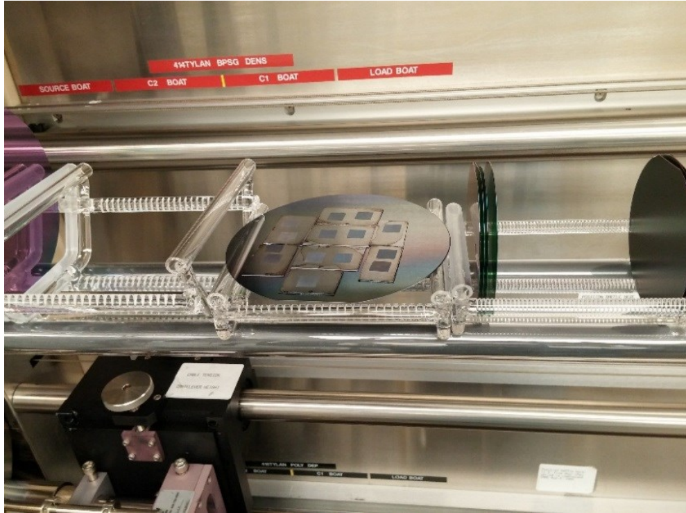
Figure 5.2 Samples loaded in the diffusion furnace
