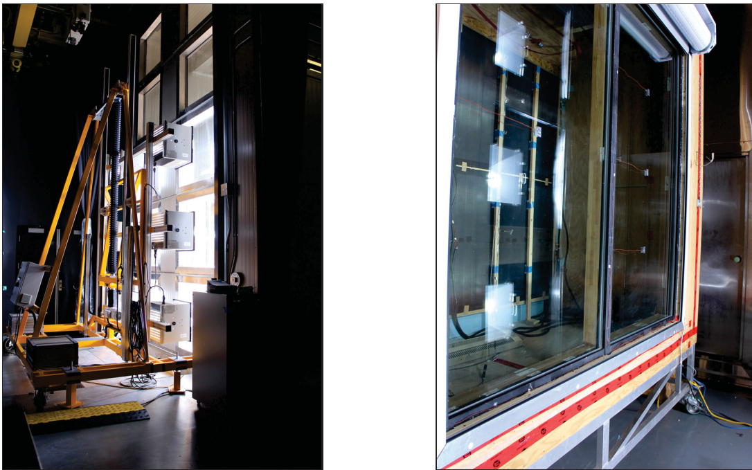
(a) Solar simulator and environmental chamber
