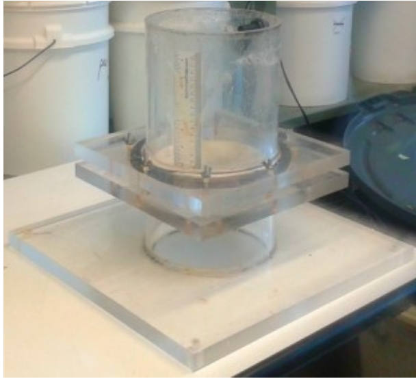
Figure 3.5 Photo of the filtration unit
