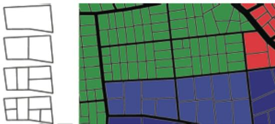
**Figure 1 :** *Left: The initial block (top) is recursive split (approximately orthogonal to the longest side) until all sub-polygons are below a land use dependent area threshold. Right: Resulting lots. Note the different sizes and ratios of the lots in residential (green) and industrial zones (blue).*
