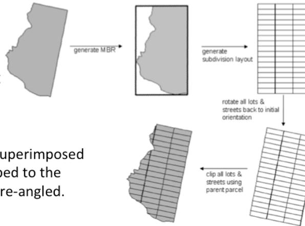
**Step 3:** The grid is superimposed onto the MBR, clipped to the block's extent, and re-angled.
