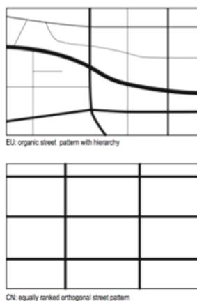
**Figure 7: Top: A hierarchical, irregular road network. Bottom: an equal, regular grid road network, Albert Speer & Partner (2012)**
