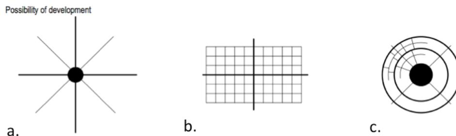
**Figure 6: Primary access structures; a. radial, b. grid, and c. circular, Albert Speer & Partner (2012)**
