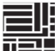
Like the gridiron, this type is orthogonal but the blocks are long and narrow and sometimes L-shaped. It favors T-intersections. This type has similar total road length as gridiron, but with fewer blocks and access
