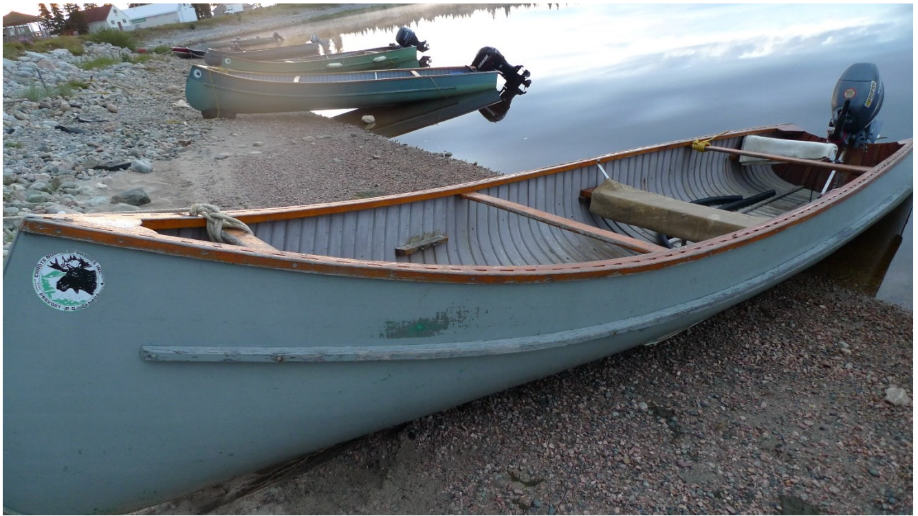
Figure 4. Freighter canoe with gasoline powered outboard motor
