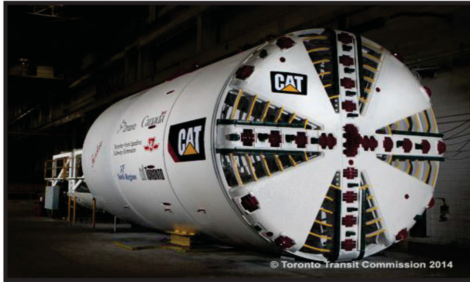
Figure 42. Tunnel Boring Machine "Torkie" (Kiewit, 2015)
