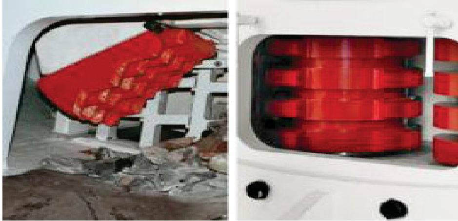
Figure 11. Jaw Crushers (left) and Drum Crushers with Agitators (right) Crush Boulders or Stones during Tunneling (Hitachizoosen, 2012)
