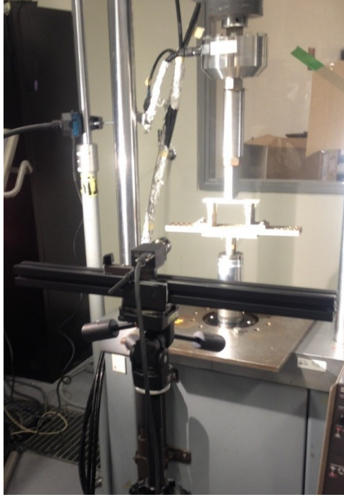
Figure 3.20: Experimental set-up for flexural fatigue test.
